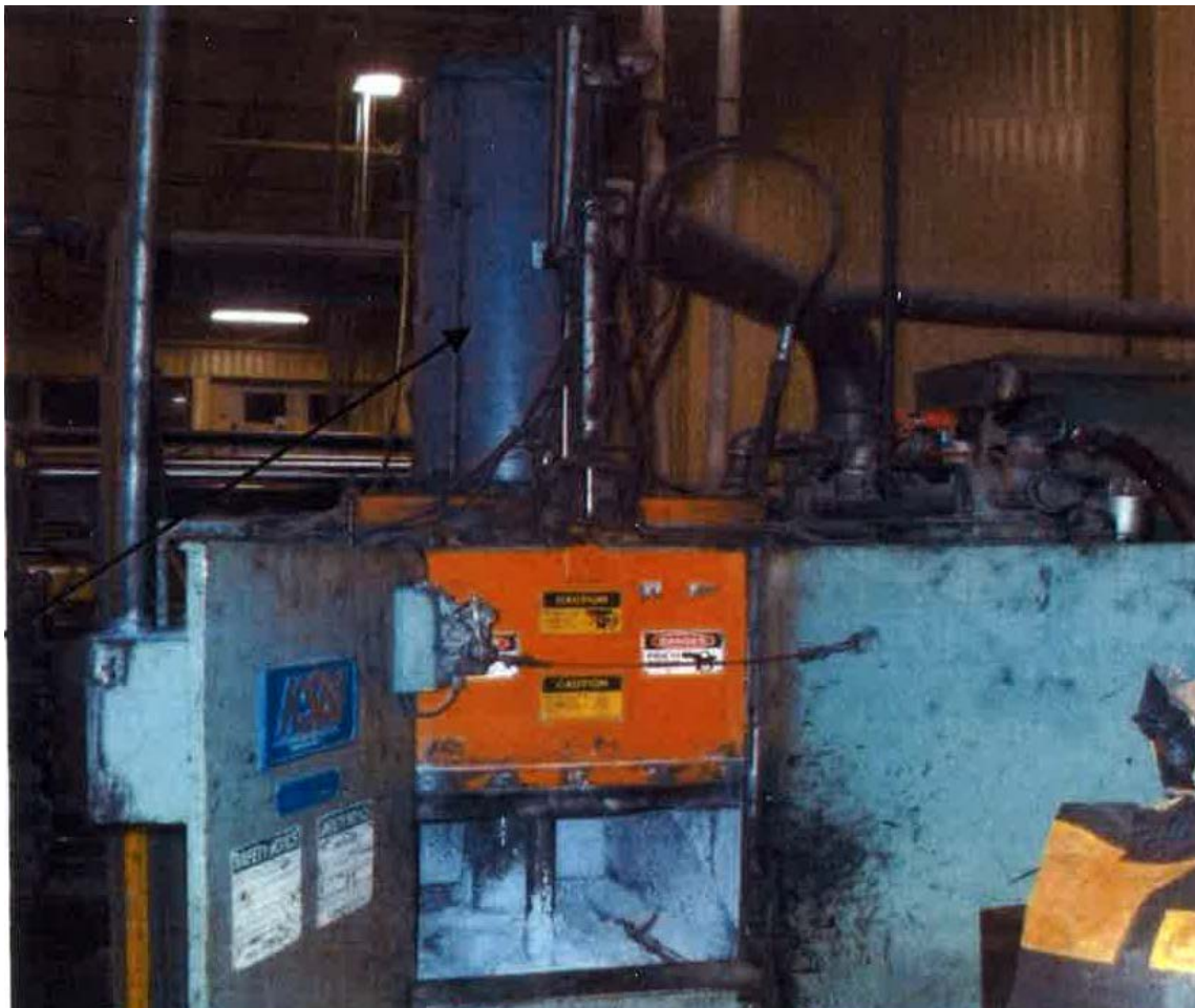
Photo 1 of 1 – Photo shows the orange mixer door and this is where the victim entered for cleaning purposes. In the photo the ram is lowered down inside the mixer hopper.
