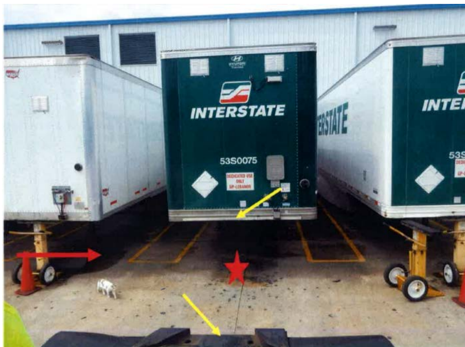
Photo 2 of 2 – The photo is a view from the rear of the truck being backed toward the trailer. The red arrow indicates the victim's direction of travel just before he was struck. The yellow arrows indicate the approximate area on the trailer and truck where the victim was pinned. The red star indicates approximate locate of the victim after the incident.
