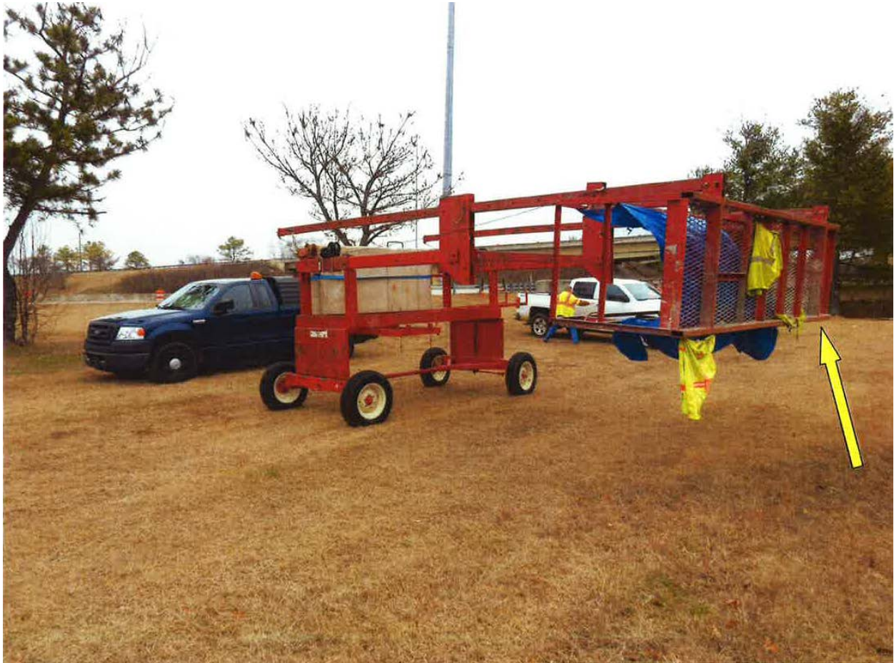
Photo 1 of 1 –The yellow arrow indicates the right-rear side of overhang buggy basket that struck the victim.
