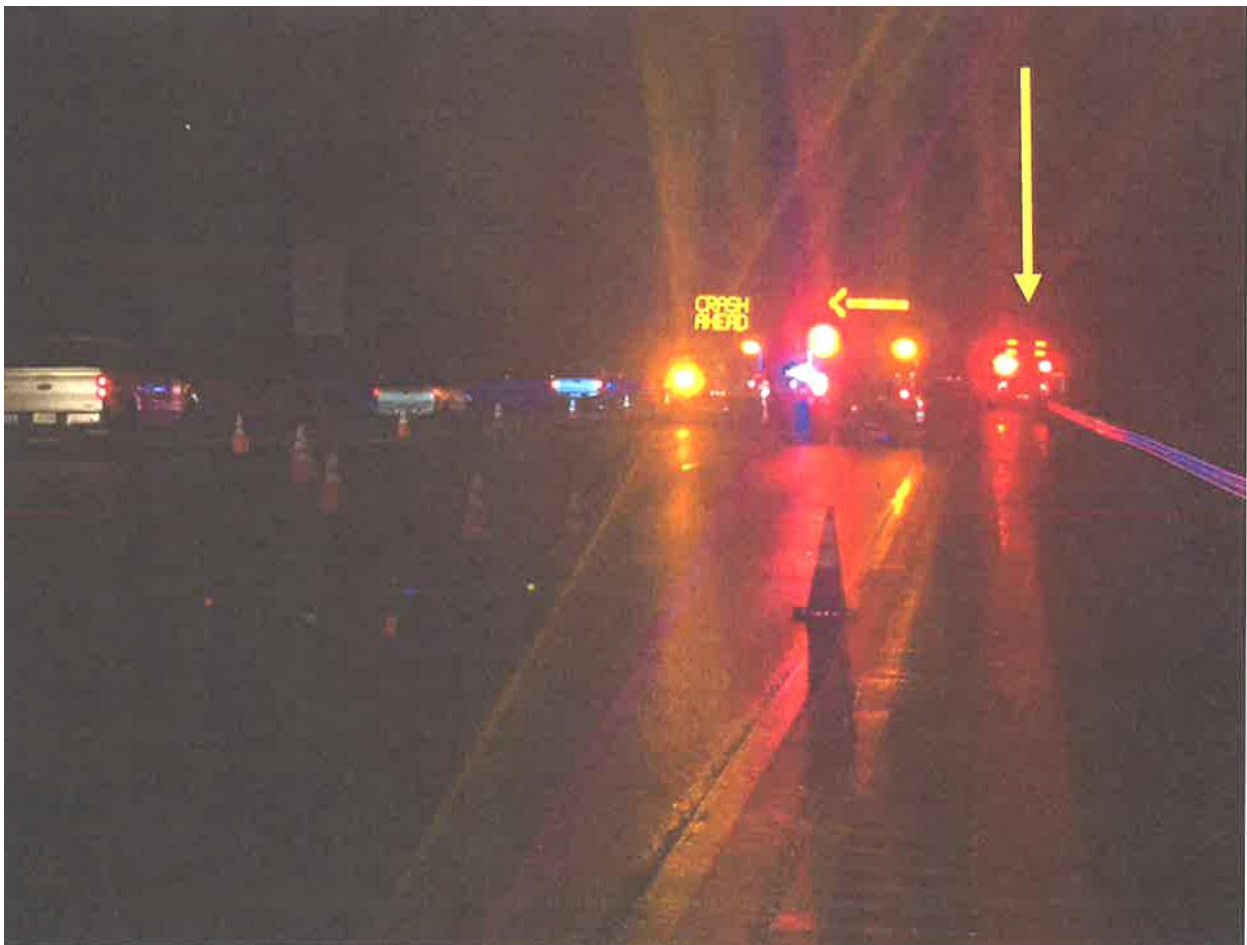
Photo 1 of 1 – The victim’s truck on the shoulder of the road (yellow arrow) with the red flashing light turned on and the message board showing the caution signal as required by the MUTCD, Manual on Uniform Traffic Control Devices.
