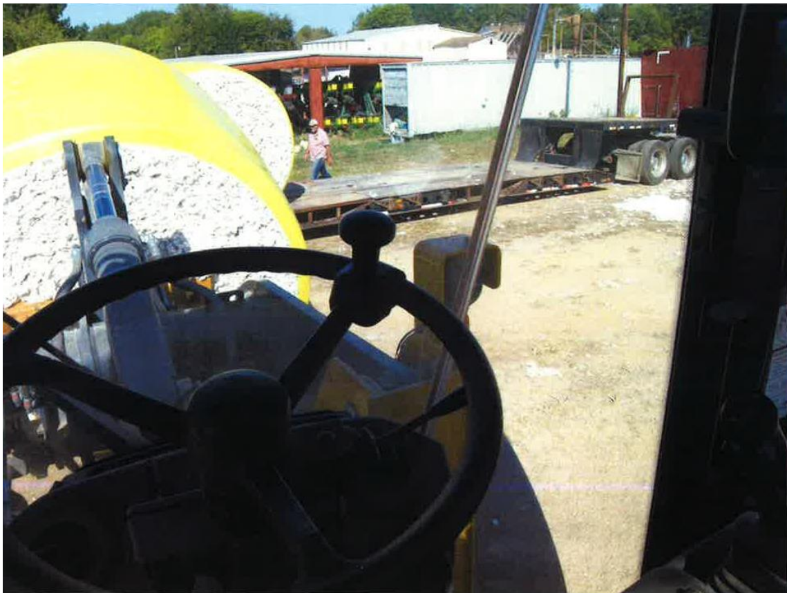
Photo 1 of 1 – View from the operator’s seat of the John Deere 544K wheel loader with a round bale of cotton loaded on the four-tine bale spear.
