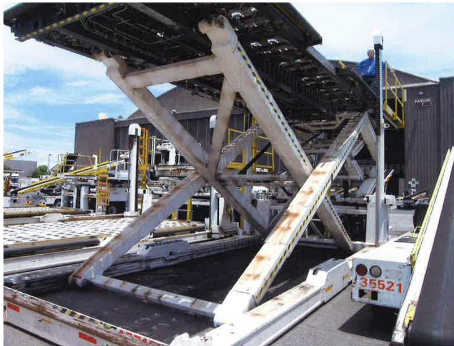
Photo 2 of 2: Cargo Loader raised for loading aircraft
