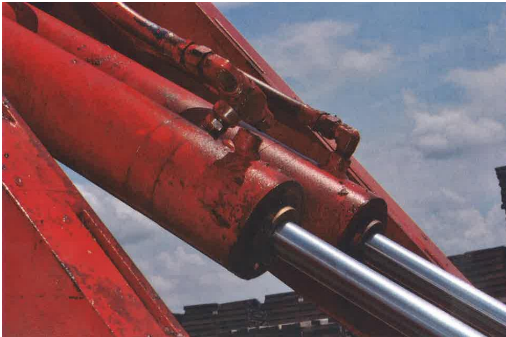
Photo 3 of 3: Broken threaded hydraulic fitting on the right side fork tilt cylinder.
