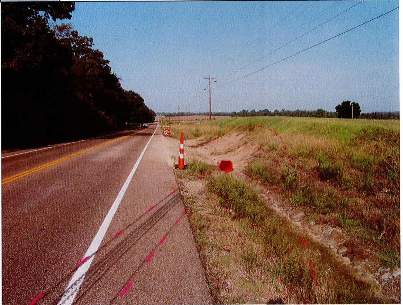
Incident site showing skid marks made by dump truck
