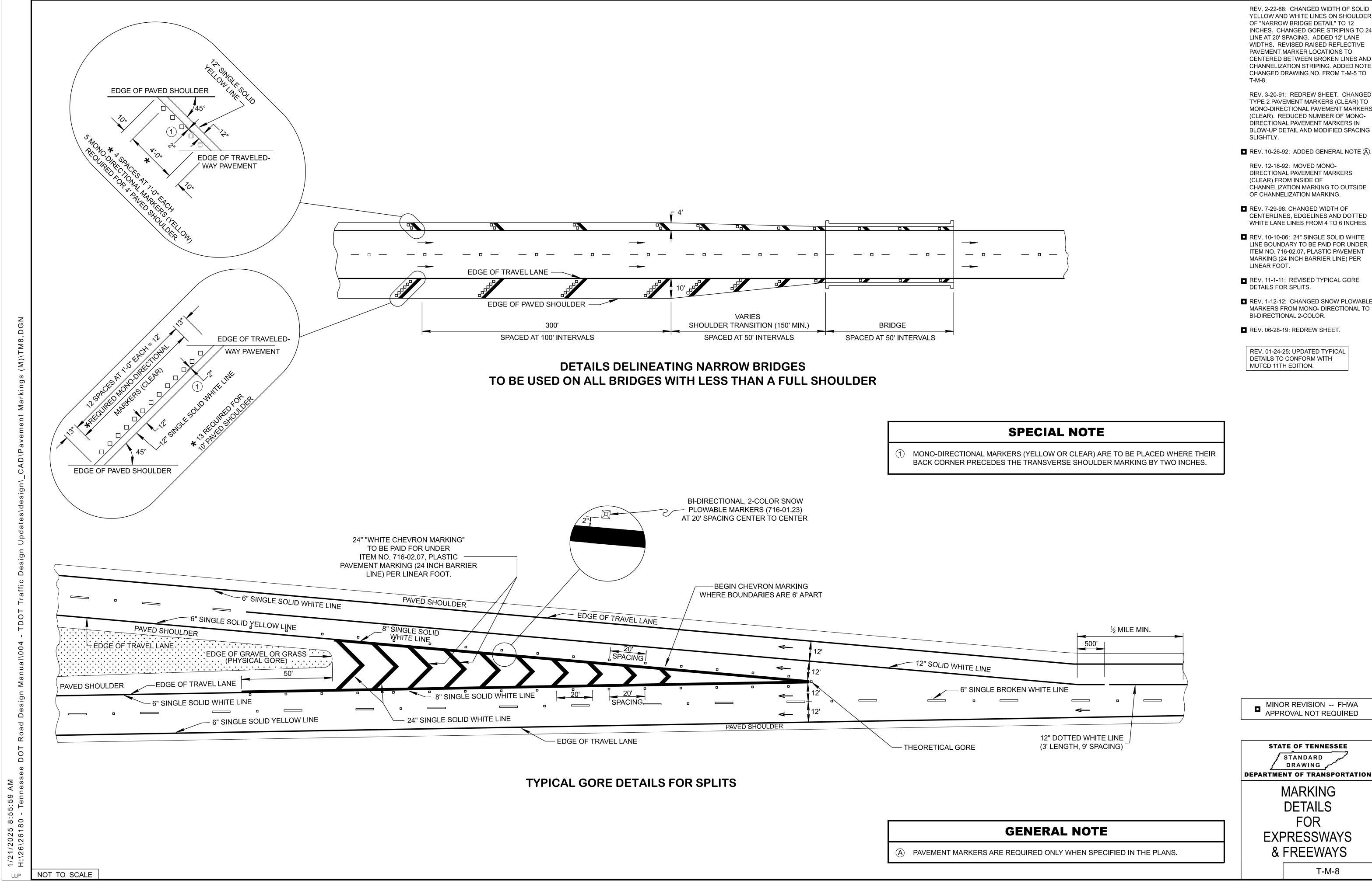
CHANGED DRAWING NO. FROM T-M-5 TO REV. 3-20-91: REDREW SHEET. CHANGED TYPE 2 PAVEMENT MARKERS (CLEAR) TO MONO-DIRECTIONAL PAVEMENT MARKERS (CLEAR). REDUCED NUMBER OF MONO-DIRECTIONAL PAVEMENT MARKERS IN BLOW-UP DETAIL AND MODIFIED SPACING
