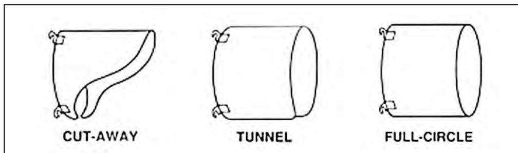
Cutaway visors, sometimes referred to as a cap or partial visors, are signal head visors with the bottom cut away. This type of signal head visor reduces water and snow accumulation and does not let birds build nests within the visor.
