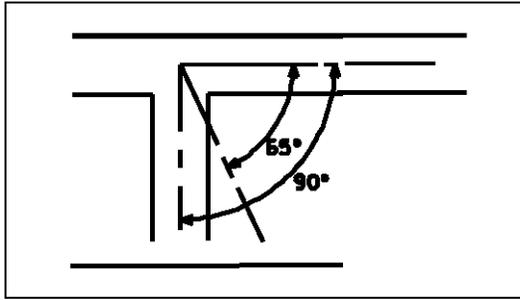
For roadway approaches with line of sight angles between 65 degrees and 90 degrees line of sight angles, use cut-away or tunnel signal head visors.
