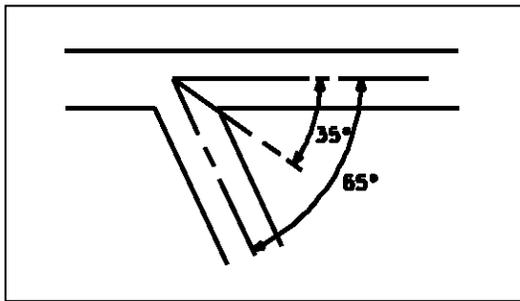
For roadway approaches with line of sight angles between 35 degrees and 65 degrees, use tunnel signal head visors or full-circle signal head visors.
