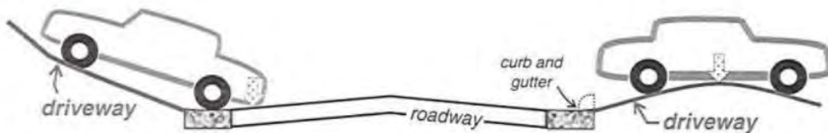
Figure 3-27: Example of Ground Clearance Issues Related to Driveway Profile.
