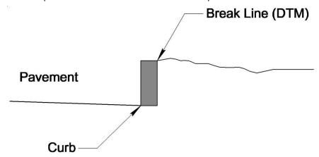
**CURB & GUTTER -** Raised edge with gutter-defining edge of pavement. Digitize the edge of pavement and the lower edge of the curb. Label as "C&G". Retaining walls have precedence over curb and gutter. **Do not** snap to the sides of curb and gutter.
