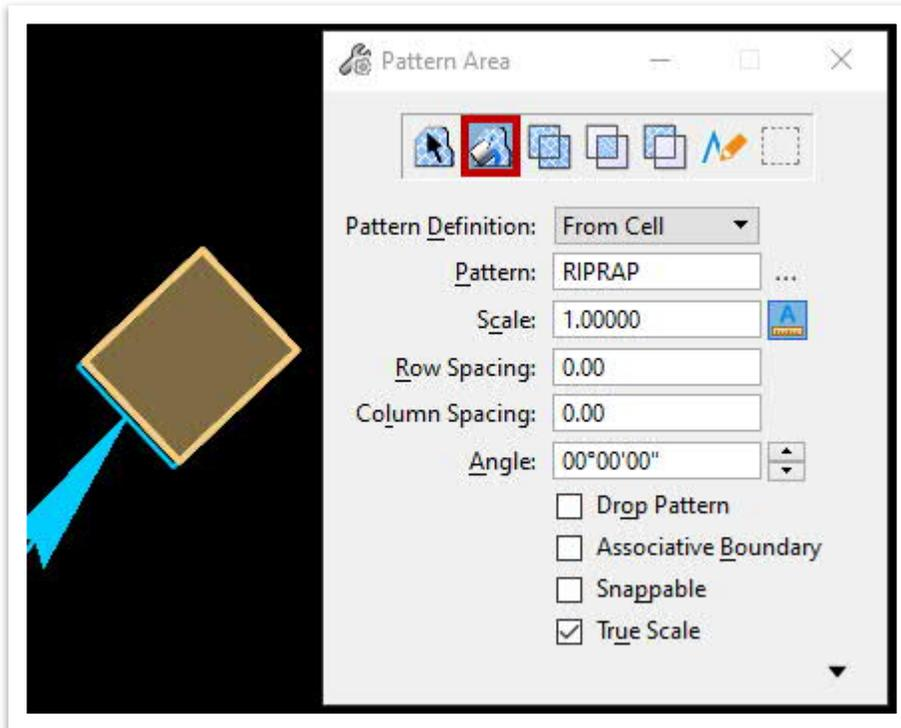
5. Left click again and notice the placement alert. Click **OK**. The riprap is now placed at the correct scale with the applicable symbology. Go ahead and turn off the **Bowling\_RipRap.dgn** reference file..
