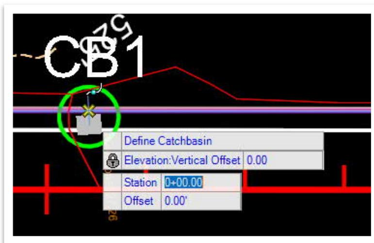
14. Move the cursor towards the location of **CB1**. Press the **letter O** on the keyboard. Notice the cursor prompt: **Select a reference element or Reset to return to command.** **Note:** If ever the Sta/Off functionality does not seem to work, you will likely need to re-select the reference element in which to base the Sta/Off by doing this step again.
