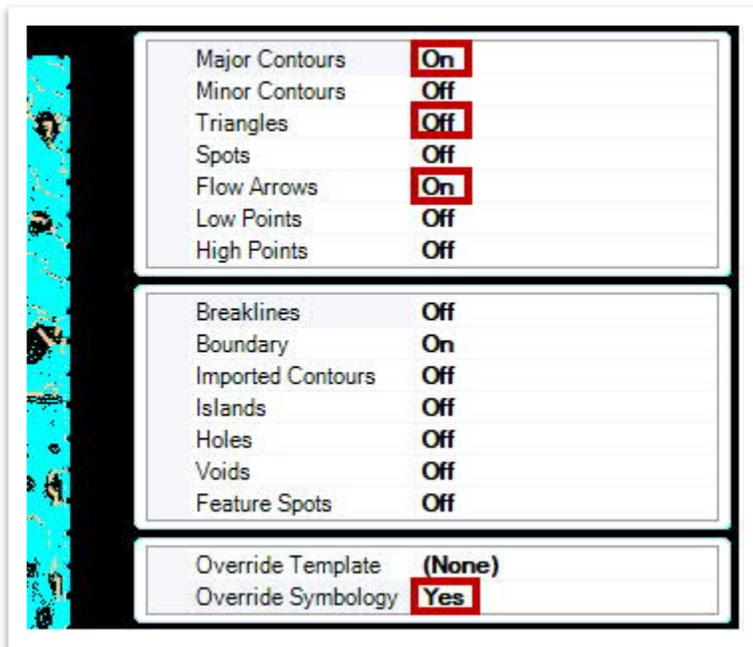
2. The density of the flow arrows is based on triangulated density of the terrain data. **Note:** If you want to change the density, you can create different terrain dgn files with various densities.
