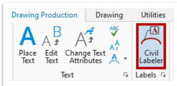
2. Within the civil labeler window, select the **Conduit Size** label (**TDOT Civil Labeler >> TDOT - Drainage and Utilities - Plan >> Proposed**). Change the **Leader** to **None** and the **Rotation** to **View Horizontal**. Leave all other predefined TDOT settings as-is. Click **Place**.
