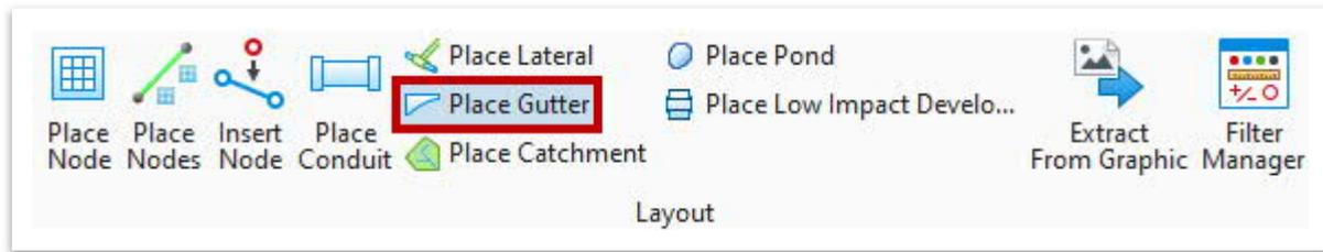
The TDOT Drainage Feature Defs.dgnlib provides **multiple** feature definitions for gutters (Figure 30). The gutter types and nomenclature correspond to TDOT’s gutter types defined within the TDOT standard drawings. The feature definitions represent the dimensions for the gutters per the TDOT standard drawings.
