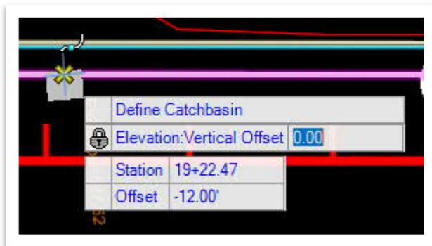
17. Move the cursor towards the location of **CB1**. Hit **TAB** once again to edit the station and offset. Key-in station **19+08.50** and offset **-15.90'** for this exercise. Hit the **TAB** or **Enter** key after each entry so that it locks in place. Left click to accept.
