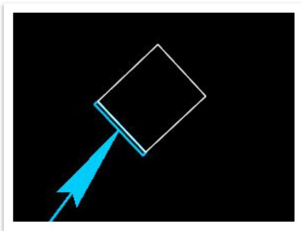
2. Now, select the **Rip Rap (Proposed)** element template (**Design >> Area Patterns >> Roadway**) so that the riprap will be placed with the correct symbology.
