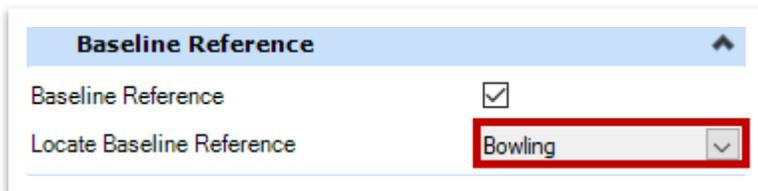
19. Next, you will be prompt to select the **Rotation Mode**. Left click to accept and a new prompt will appear asking you to **Locate Reference Element for Rotation**. Select the **Bowling** centerline and hit **Enter**. Left click to accept the rotation. Alternatively, you could select the Rotation Mode in the **Place Node** dialog box. In this exercise, we are checking the Rotation box and leaving it at 90 degrees. Left click to accept and then hit **ESC** to clear the tool.
