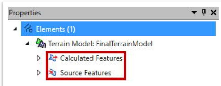
Under **Calculated Features** you can control the display of the flow arrows, high and low points, spots, and triangles, plus the contours (Figure 12). Each feature has a designated level so that the user can turn each feature on and off, as necessary.
