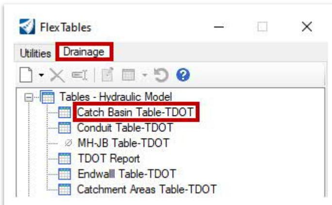
3. Within the **Catch Basin Table-TDOT** flex table, update the CB1 **Inlet** type to **Type 12 - 48x48** and then close the window.
