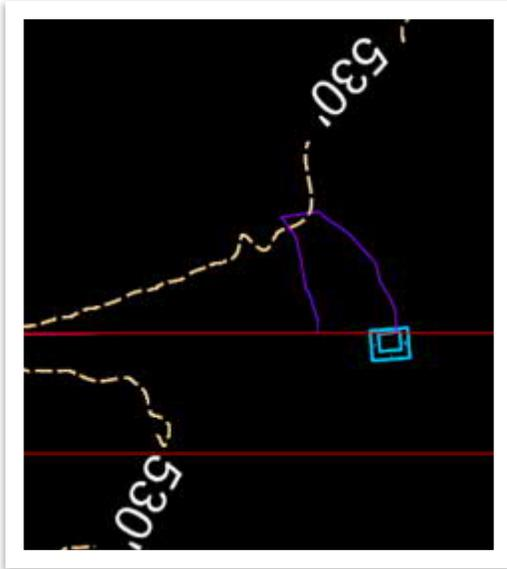
5. Place a second catch basin within the delineated area of the first catch basin using the same structure type and catchment.
