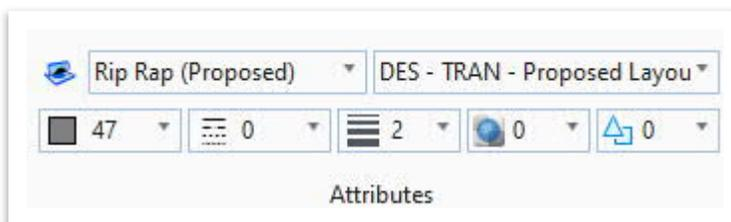
3. Next, open the **Pattern Area** tool. The quickest method is to use the search ribbon in the upper right corner of the ORD interface. **Note:** You could also find the tool in the **Drawing** workflow under **Annotate >> Patterns**.
