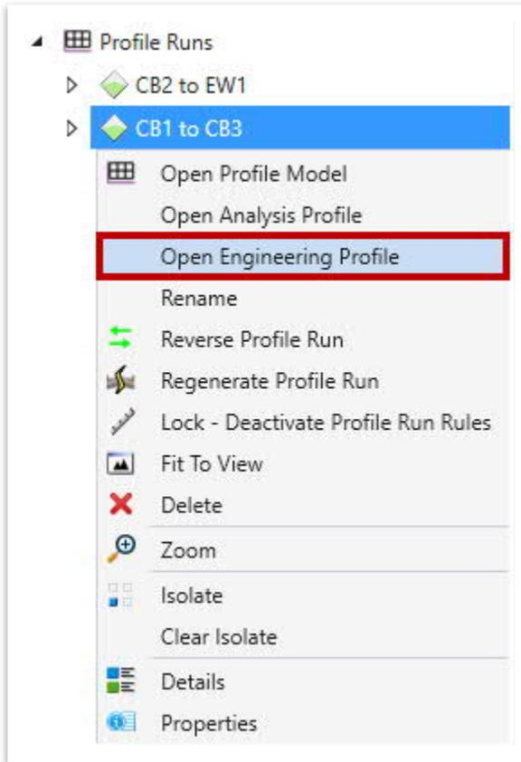
11. In the **Engineering Profile** window, review the **Nodes, Conduit, Ground Elevations, Inverts, etc.** to verify if the inlets and pipe are connected correctly in the direction of flow, along the storm drain. **Note:** You may review the engineering profile of the other profile run (**CB2 to EW1**) in the same manner.
