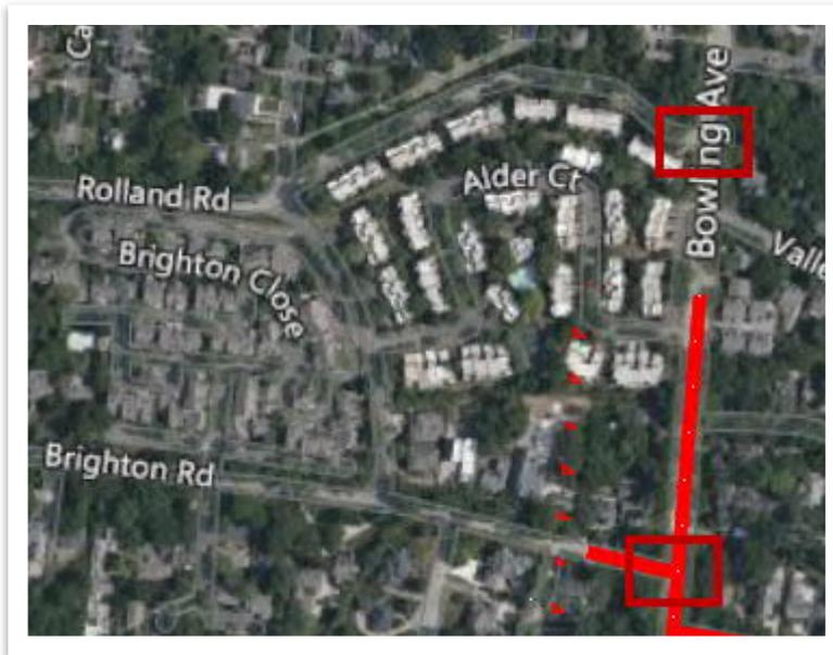
5. Since there is not any geometry linework at the Rolland Rd intersection, we need to draw a line so we can snap to the location easier. Open the **Place Smart Line** tool (**Drainage and Utilities >> Drawing >> Placement**) and draw a line like what is shown below.
