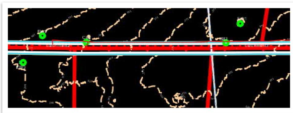
3. We will now place catch basins at the approximate locations shown. **The location of CB3 is a sag point on the roadway.** Before we place any catch basins, it is recommended to review the **centerline profile**. Select the **Bowling centerline** and open the **Open Profile Model** tool. It can either be accessed within the heads-up display (2<sup>nd</sup> icon) or within the ribbon under **Drainage and Utilities >> Utilities View >> Drawing Views**.
