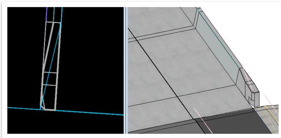
29. Repeat Steps 26-28 to place the bridge end in the remaining three corners, making sure to use the corresponding feature definition for each orientation. **Note:** **Start** and **end** are flipped for the **Left** side as the start/end is based on travel direction (i.e., the SW corner will use the **Left End** feature definition).
