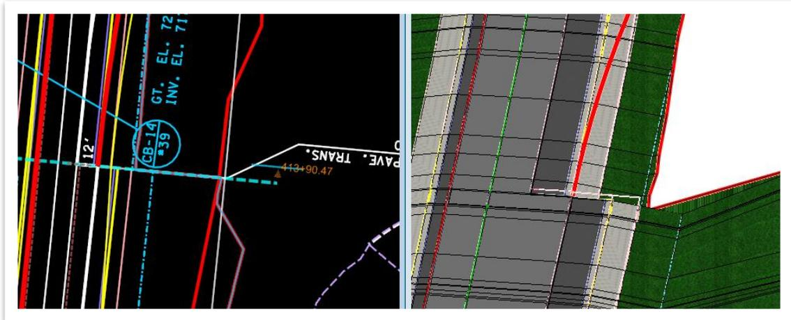
7. Next, we need to turn the mainline corridor **shoulder** off. Open the **Create Parametric Constraint** tool (**OpenRoads Modeling >> Corridors >> Edit >> Edits**) and select the **I65** corridor. Then, select the following settings.
