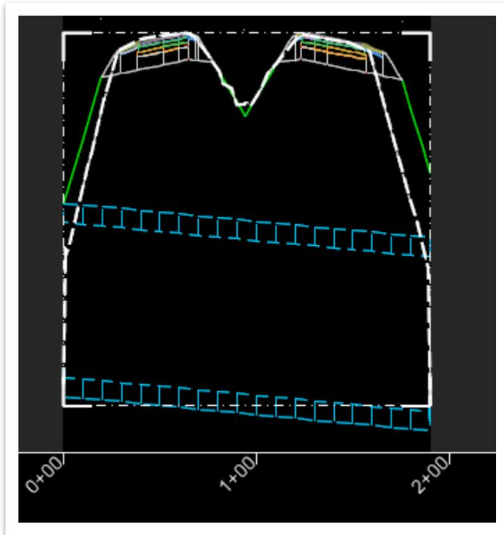
11. We need to determine the maximum height available for a new box culvert should the current size be deemed insufficient. This scenario has a maximum of **16.7'** available. Assuming a **6"** curb lip and **10"** ST value, the max standard height of this structure could be **14'**. We will confirm the size of the box culvert in the next exercise.
