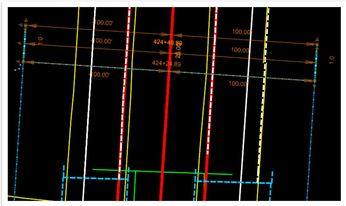
12. Then, open the **Line Between Points** tool (**OpenRoads Modeling >> Geometry >> Horizontal >> Lines**) and connect the two offsets.
