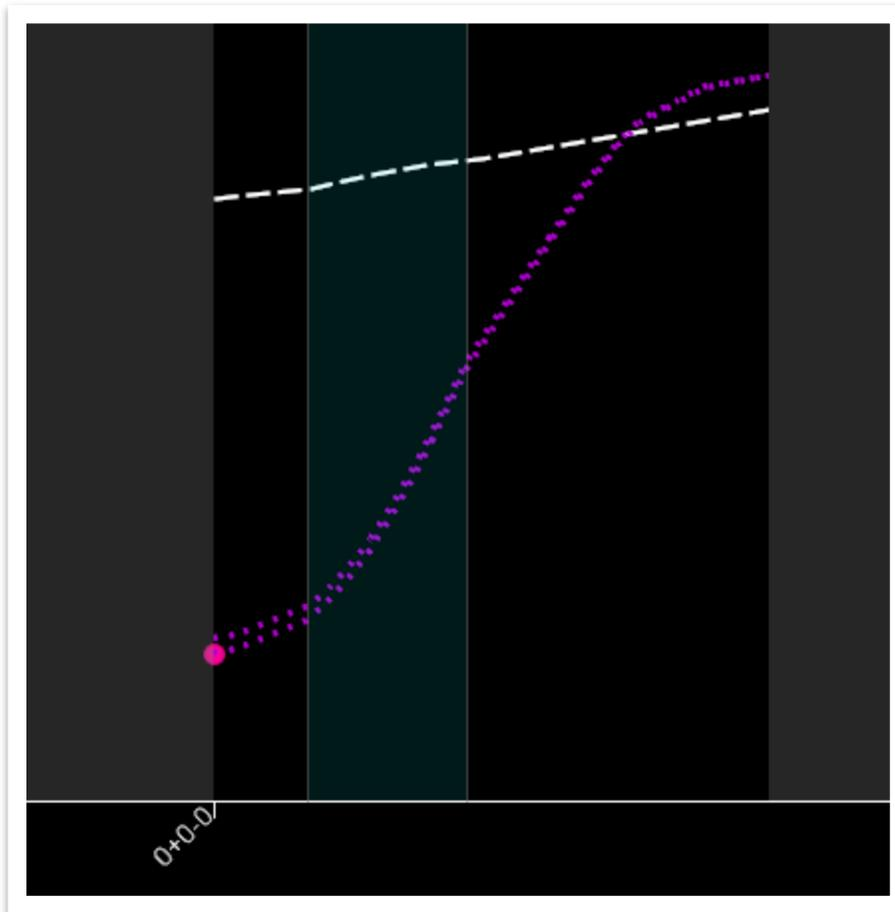
26. Currently the driveway EOP's do not intersect with the sidewalk back top of the driveway civil cell. We will need to transition the driveway EOP's profile to line up with the sidewalk back top. Go ahead and select the **Prop EOP - Driveway - CTRL** feature definition (**Linear >> Roadway >> Model Control - 2D plan >> EOP**).
