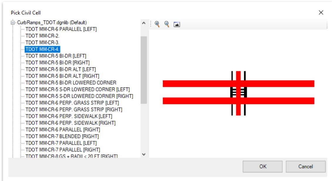
30. Follow the prompts and select the top **CR Flowline** (1), the top **CR Back Top** (2), the bottom **CR Flowline** (3), the bottom **CR Back Top** (4), and then the orange **Ramp Centerline** (5).
