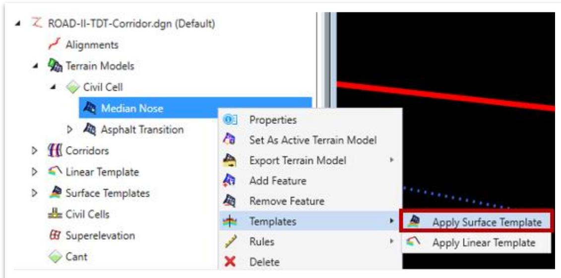
47. Select the **SURFACE - CONC. MISC.** template (**Linear Templates >> Civil Cells >> Surface**) and left click through the prompts to apply the surface template.
