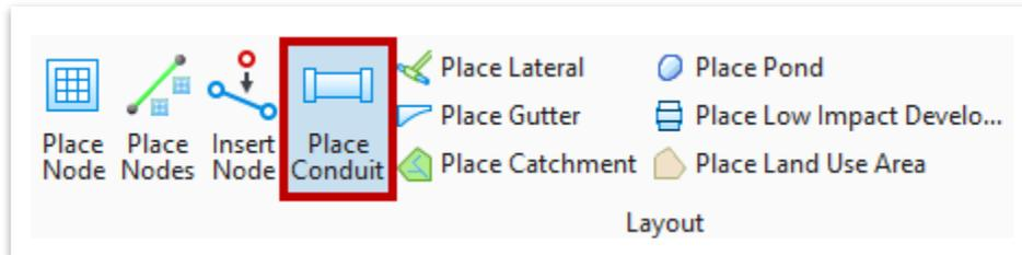
9. Select the **RCBC** feature definition (**Conduit >> StormWater >> Culvert Pipes >> Proposed**) and set the **Description** to **8x8**. **Note:** If the **8x8** option is not available under the **Description** drop-down, close the file and clear your user preferences.
