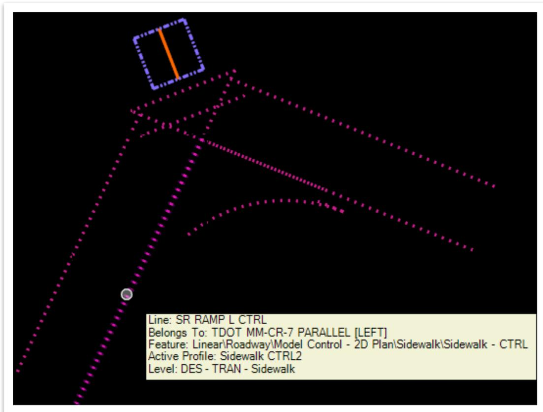
26. Go ahead and change the slope of the profile from 8.33% to **3.5%**. Notice the ramp has extended but the **R** side of the ramp is still sloped at 8.33%. This is because of the complexity of the civil cell, where both **CTRL** element slopes will need to be manually adjusted. The slopes need to be the same, but this civil cell is one of the exceptions where the mainline and sideroad ramp slopes can be different.
