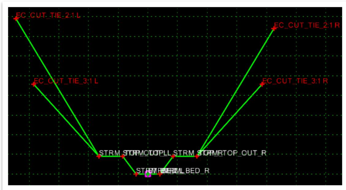
13. Now, we will create a **New Corridor** using the stream centerline. Open the **New Corridor** tool (**OpenRoads Modeling >> Corridors >> Create**). Within the **Create Corridor** dialog box, select the **Preliminary Design** feature definition and name the corridor **STRM 2**. Select the proposed stream centerline, **right** click to accept the active profile, and then **left** click to accept.
