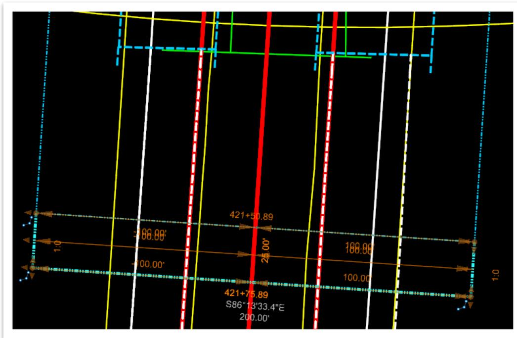
14. There should now be **three** shapes that are not complexed together: one bridge, one approach slab at the beginning of the bridge, and one approach slab at the end of the bridge. The additional **25** feet is for the approach slab template drop.
