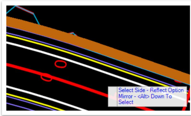
10. The template has now been placed in the model. Go ahead and delete the dummy element created in Step 5. Now, we need to edit the template to match the proposed special ditch configuration. Open the **Edit Template Drop** tool (**OpenRoads Modeling >> Corridors >> Edit**) and select the **special ditch** template drop.
