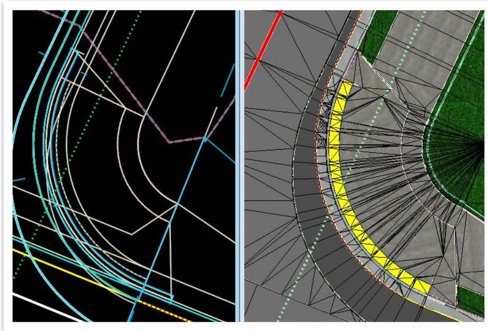
20. Zoom in and notice once again that the sidewalks have been tapered and adjusted to meet the back of the civil cell ramps. This is because the civil cell is built with the maximum slope of **8.33%** and the sidewalk needs to be widened to match the civil cell.
