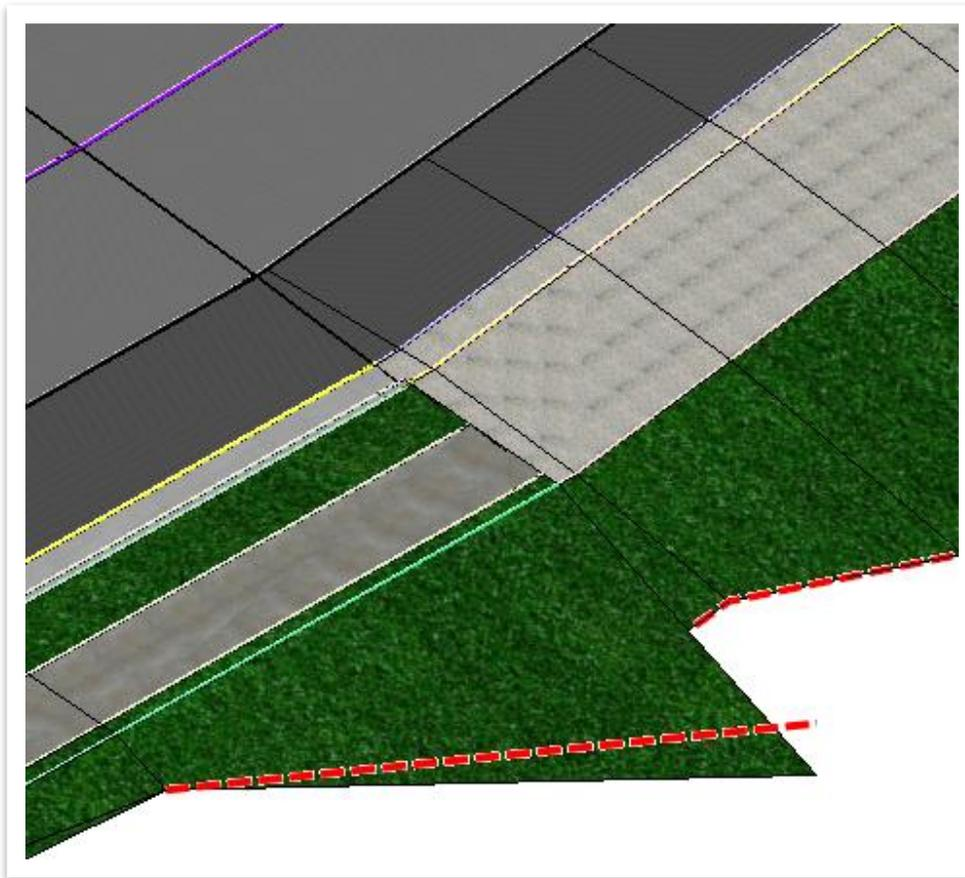
19. Repeat Steps 11-18 to place the same linear template for the left side of the roadway. The **start** and **stop** locations for this template drop will be Stations **83+53.23** and **85+29.49** respectively.
