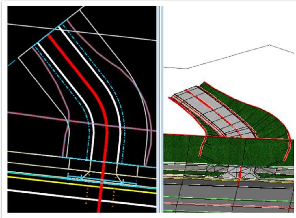
18. Notice that the mainline corridor is **overlapping** with the driveway corridor. Open the **Add Clipping Reference** tool (**OpenRoads Modeling >> Corridors >> Miscellaneous >> Corridor Clipping**). Select the mainline corridor and then the driveway corridor as the clipping reference. **Right** click to complete the clipping.
