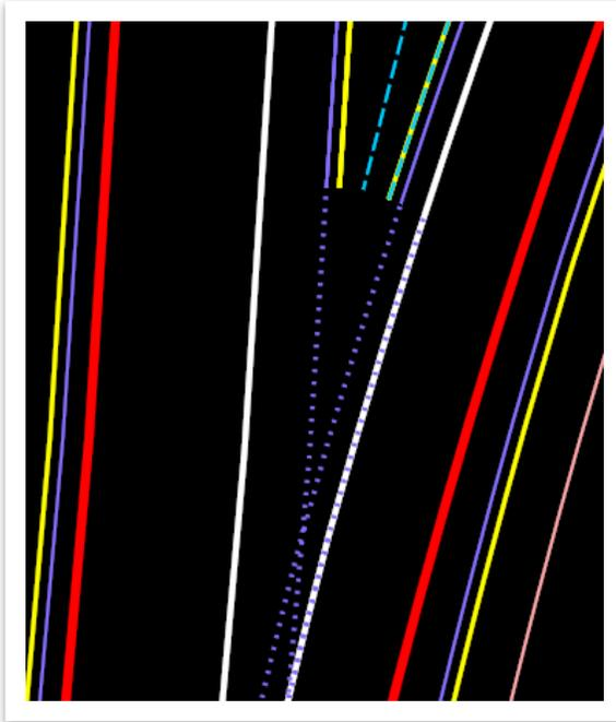
45. Now, we need to create the **curved nose** of the paved gore. Open the **Simple Arc** tool (**OpenRoads Modeling >> Geometry >> Horizontal >> Arcs >> Arc Between Elements**). Select the two **EOP - CTRL** lines that were offset in the previous step and then place the arc near the end of the shoulder lines. Set the Trim to **Both**.
