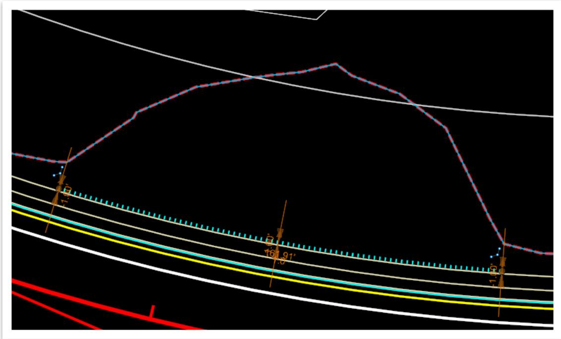
13. Next, open the **Apply Linear Template** tool (**OpenRoads Modeling >> Model Detailing >> 3D Tools**) and select the line that was just placed.
