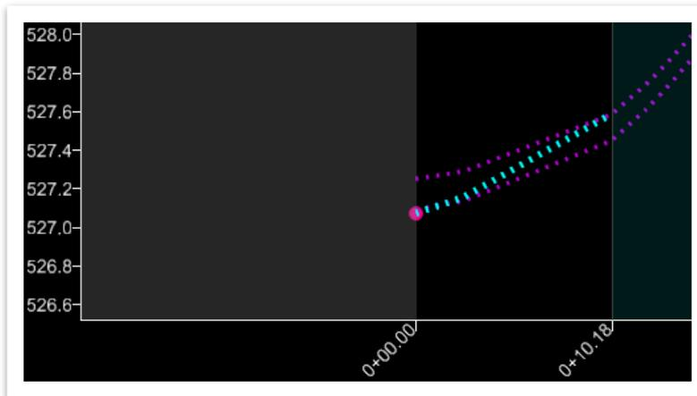
30. Now select the **VARIABLE SLOPE L** profile line and open the **Properties**. Within the properties under the **Profile By Projecting 3D Element Slope Rule** header, change the **Start Reference Distance** to Station **0+10.00** and the **Start** and **End Slopes** to **0.00%**.
