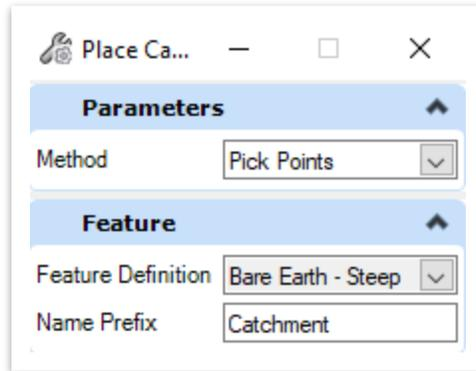
20. **Left** click to accept the **Method** and then draw a **complete shape** anywhere near the ditch **begin** node around Station **162+50.00**. **Right** click once the shape is complete. **Note:** Your shape does not need to match exactly. It can be any closed shape with any area. The drawn area will be ignored, and we will input a pre-determined drainage area value.
