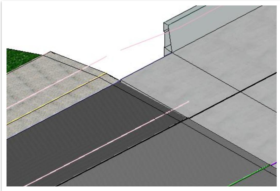
24. Repeat the process for the additional **three** corners of the bridge, using the **RIGHT\_BARRIER\_CTRL** constraint for the right side of the template. The **Start** and **Stop Stations** will change accordingly on the north side of the bridge to **424+24.89** and **424+42.89**.
