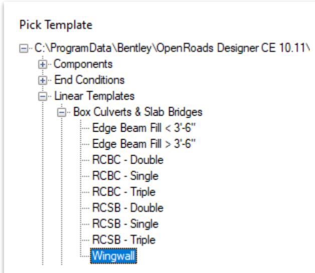
18. Select the **upstream right** wingwall geometry to apply the template. Toggle on **Lock To Start** and **Lock To End** and then click through the prompts to accept. When prompted which side to place the template, select towards the center of the box culvert.
