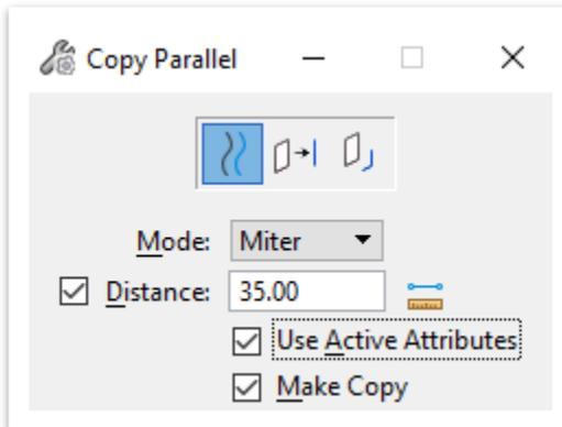
18. Select the **LBL** and **left** click to the outside of the stream to offset the LBL by 35'. Then, select the **RBL** and **left** click to the outside of the stream to offset the RBL by 35'. Once complete, turn off the **ROAD-II-HEC-Survey.dgn** reference file once again to view the stream bank lines. **Note:** If necessary, you can check and remove any extra vertices or kinks in the overbank lines to smooth them out. For this exercise, the overbank lines were not altered.
