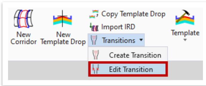
Within the **Edit Transition** tool, the **first window** allows you to delete automatic links and create new links between points in the two template drops (Figure 12).
