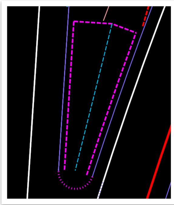
51. Set the **Feature Type** to **Boundary**, the **Edge Method** to **None**. Set the **Feature Definition** to **Civil Cell** and the terrain **Name** as **Gore Aggregate**.
