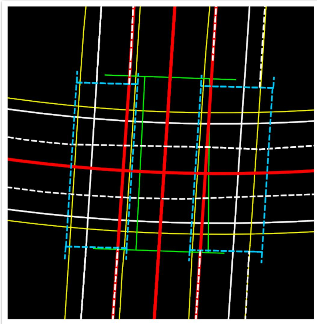
7. Select the **Clipping Boundary - Bridge** feature definition (**Linear >> Roadway >> Model Control - 2D Plan >> Clipping**).
