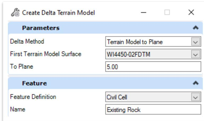
15. **Left** click to accept and notice a new **existing rock** terrain surface has now been created **5'** below the original existing terrain. Within the new terrain, go ahead and turn off the **triangles**, if not already off.
