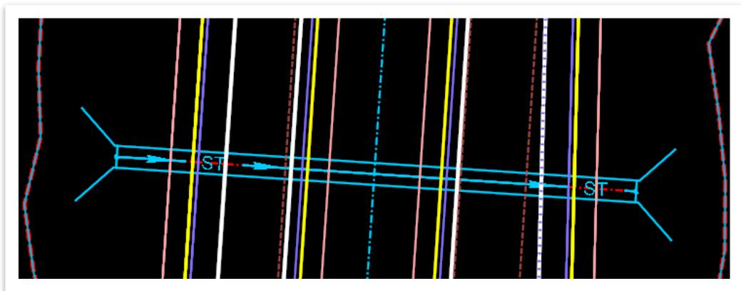
3. Within the **ROAD-II-BC-Drainage Model.dgn** reference file, turn off all levels other than the **DES - MODEL - Lines - RCBC - Centerline** level. Locate the box culvert centerline and then open the **Apply Linear Template** tool (**OpenRoads Modeling >> Model Detailing >> 3D Tools**).
