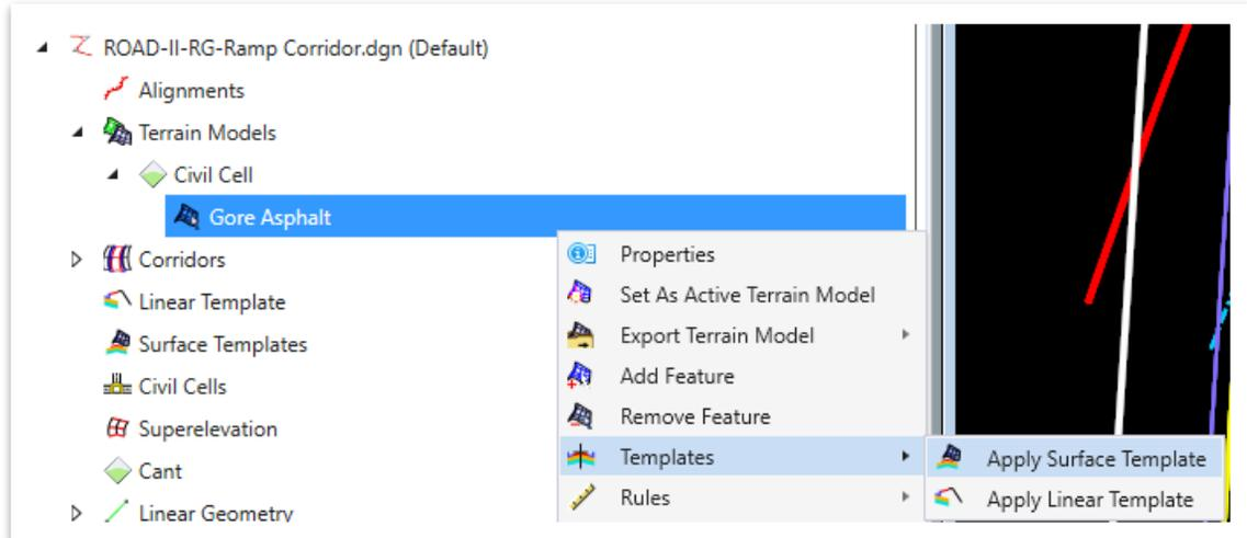
49. Select the **SURFACE - SHOULDER** template (**Linear Templates >> Civil Cells >> Surface**). Toggle off **Apply External Clip Boundary** and then click through the remaining prompts to apply the surface template.
