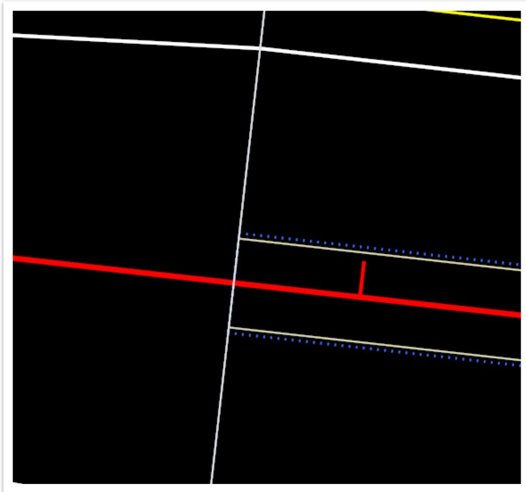
24. Select the **CTRL** lines that were just placed and open the **Properties**. Within the properties under the **Profile By Projecting 3D Element Simple Slope Rule** header, change the **Slope** to **-2.00%**.
