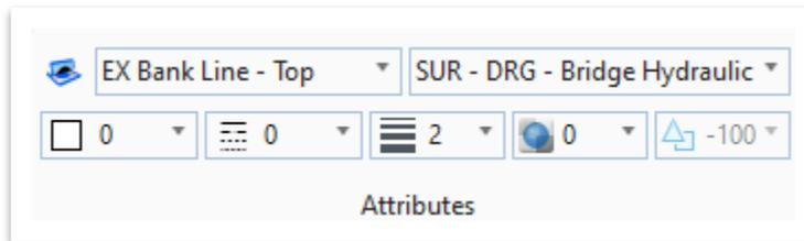
14. The left bank line (**LBL**) and right bank line (**RBL**) are established from the stream CL facing downstream. For this exercise, the LBL will be on the left (northwest), and the RBL will be on the right (southeast). Open the **Place SmartLine** tool once again (**OpenRoads Modeling >> Drawing >> Placement**) and select the settings shown below.
