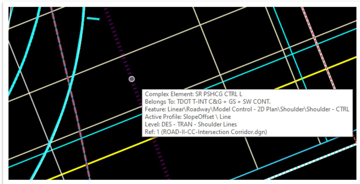
Civil Cells are placed using the **Place Civil Cell** tool (**OpenRoads Modeling >> Model Detailing >> Civil Cells**) (Figure 6).
