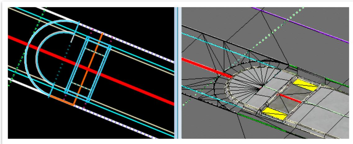
32. Notice that there is a clipping issue with the mainline (the vertical gray rectangle on the top side of the curb ramp). To fix the issue, open the **Place Shape** tool (**OpenRoads Modeling >> Drawing >> Placement**) and place a small shape around where the clipping issues are in the **2D** view. The shape should cover the median flowline (blue line) across where the civil cell is.
