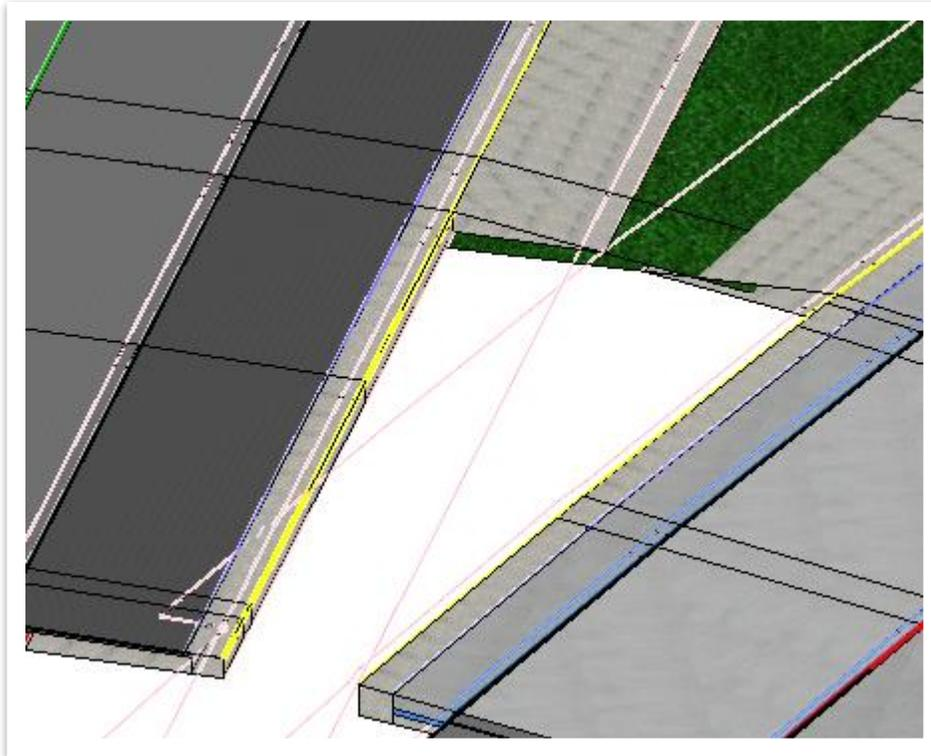
31. We will now draw the controlling lines for the two surface templates we are going to create. Open the **ROAD-II-RG-Ramp Corridor.dgn** file once again. Select the **Special Ditch - EDGE - IN - CTRL** feature definition (**Linear >> Roadway >> Model Control - 2D Plan >> Special Ditch**).
