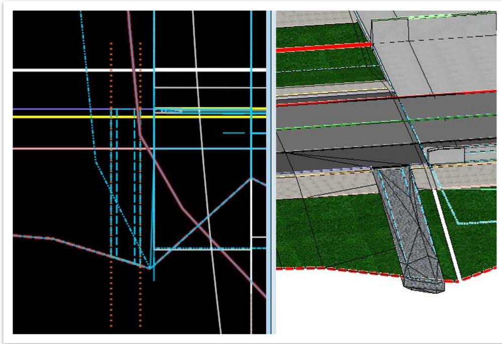
8. Zoom in to the bottom of the civil cell and locate the **orange** matchline handle slightly offset from the tie slope line. Changing the location of this handle changes the breakline of the civil cell and allows it to match the standard drawing, where it can move up to **5'** from the end of the ditch. **Note:** You can select the outside lines on the civil cell and profile them to match the slopes of the fill, if desired.
