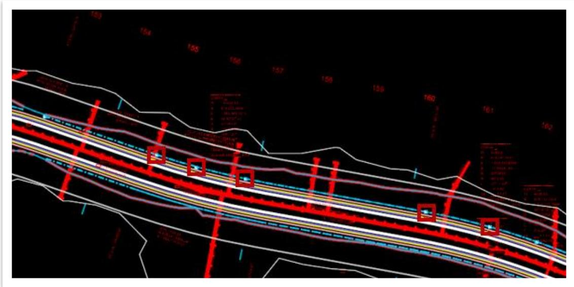
11. Before placing conduit between the nodes, we need to confirm the standard ditch configuration from the **proposed** corridor cross sections. Switch back to the **OpenRoads Modeling** workflow. Open the **Open Cross Section View** tool (**OpenRoads Modeling >> Corridors >> Review >> Dynamic Sections**). Select the **proposed** corridor and open in any view. **Note:** If you select the alignment instead, the temporary dimension labels in the upcoming steps will not work.
