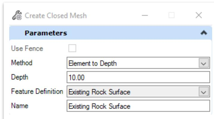
18. **Left** click to accept the **Method**. When prompted for the **Top Surface Element**, select the **Existing Rock Surface** terrain created earlier in the exercise. When prompted to select the **Boundary Surface Element**, select the **offset terrain**. **Left** click through the remaining prompts to accept.
