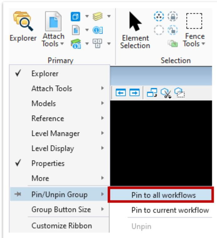
17. Now that the large **Primary** group is pinned to every tab, you can remove the simplified **Primary** tool group that was in most of the tabs by default. **Right** click on any tool group and select **Customize Ribbon**.
