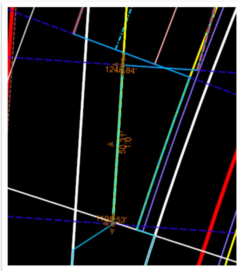
34. Within the feature definition toolbar, make sure **Create 3D Automatically** is still toggled on. Open the **By Angle From Element** line tool (**OpenRoads Modeling >> Geometry >> Horizontal >> Lines >> Line From Element**).
