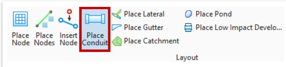
6. Select the **Side Drain RCP** feature definition (**Conduit >> StormWater >> Culvert Pipes >> Proposed**). Place a **30" RCP** connecting the endwalls under both driveways to complete the relocated stream model. **Note:** You should place conduit in the **direction of flow**, which is opposite the mainline stationing.
