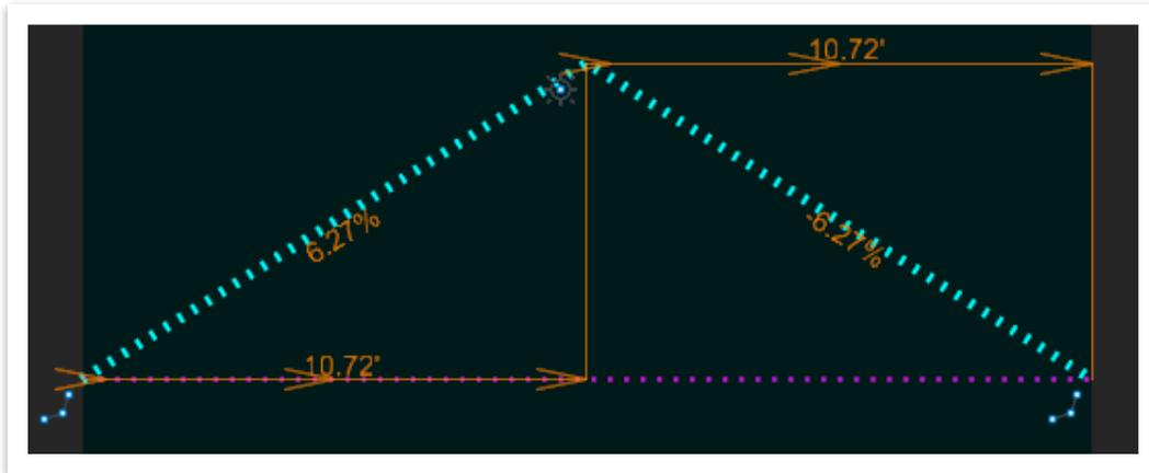
33. Now, open the **Apply Linear Template** tool (**OpenRoads Modeling >> Model Detailing >> 3D Tools**) and select the arc.
