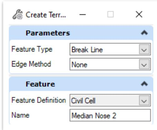
42. Within the **Explorer**, **right** click on the **Median Nose 2** terrain just created (**OpenRoads Model >> Terrain Models >> Civil Cell**) and select **Apply Surface Template**.
