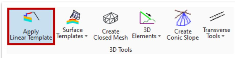
37. Select the **Median C&G** linear template (**Linear Templates >> Civil Cells >> C&G**) and click **OK**.
