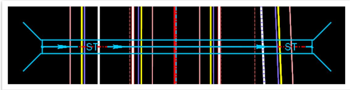
45. Since we know that the existing box inverts work, we will need to create a profile for the box culvert. Open the **STR-5 RCBC** profile and delete the **3D cut** if it is still present, by hovering over the 3D cut border and selecting the red X in the heads-up display. The profile should just have the active terrain in it. Select the **RCBC - Centerline** feature definition (**Linear >> Roadway >> Drainage >> RCBC**).
