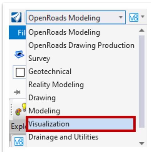
4. Open the **Stencil 2D Elements on 3D Geometry** tool (**Visualization >> Home >> Utilities**).
