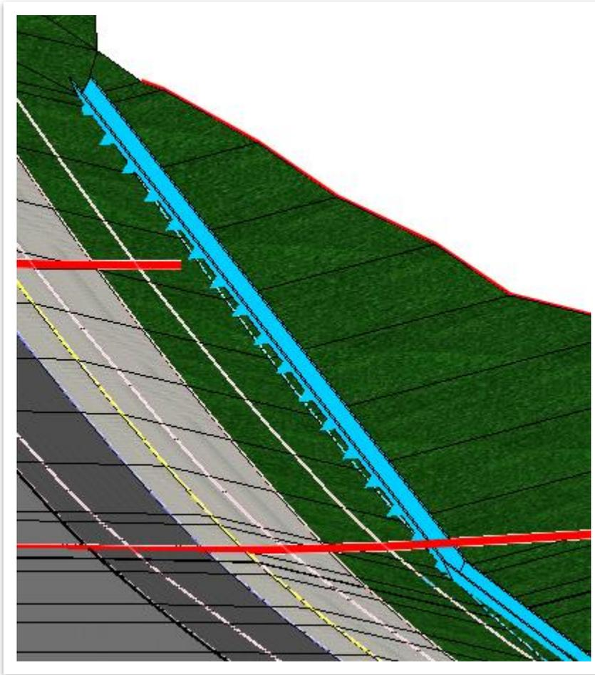
18. Lastly, we need to define a **catchment area** and input a defined **acreage** and **time of concentration**, so we can run the analysis. Open the **Place Catchment** tool (**Drainage and Utilities >> Layout >> Layout**). Turn off the **ROAD-II-SD-Corridor.dgn** reference file.
