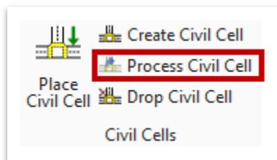
The **Drop Civil Cell** tool (Figure 9) will disassociate all geometry within the civil cell, allowing each line to be selected individually. This is useful if the civil cell is going to be heavily edited and modified. Once this tool has been used, elements will have to be **individually deleted**. Therefore, it is recommended to not drop a civil cell after placement unless absolutely required.
