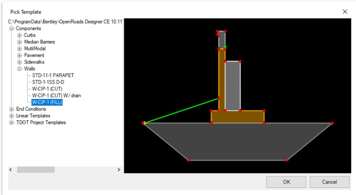
15. **Lock** to **start** and **end** and place the orange object on the **inside** of the road and click through the prompts to accept.
