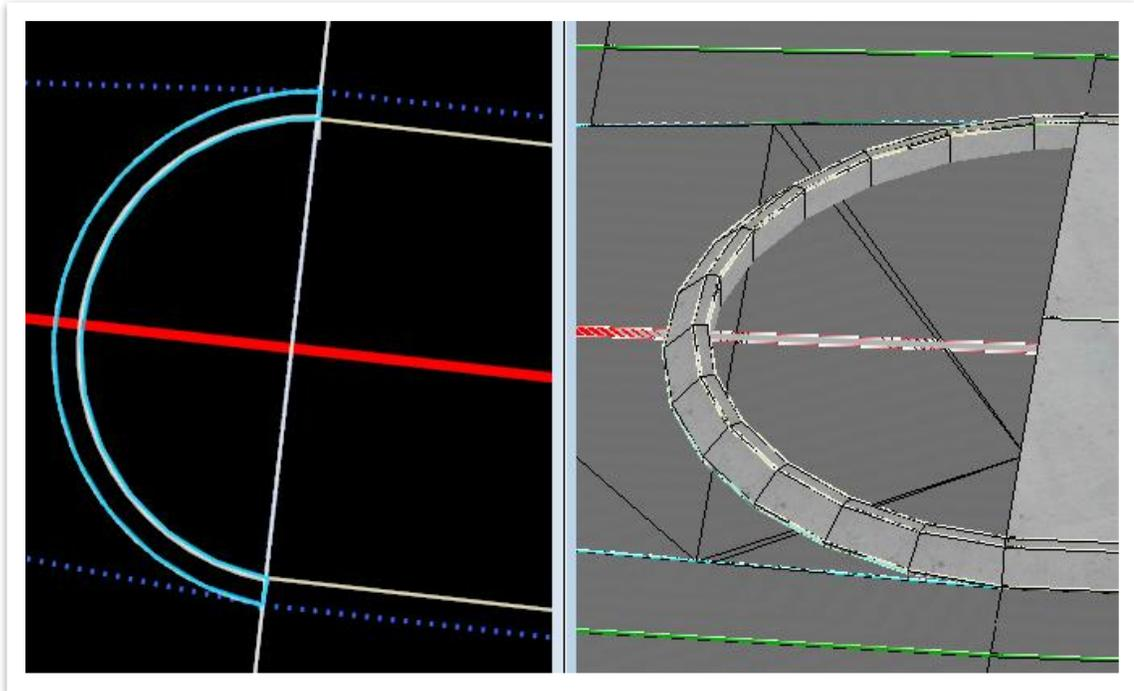
40. Open the **Line Between Points** tool (**OpenRoads Modeling >> Geometry >> Horizontal >> Lines**) and draw a line from the inside edge of the linear template to the other, snapping to the arc (**CR\_BACK\_TOP\_RM**).
