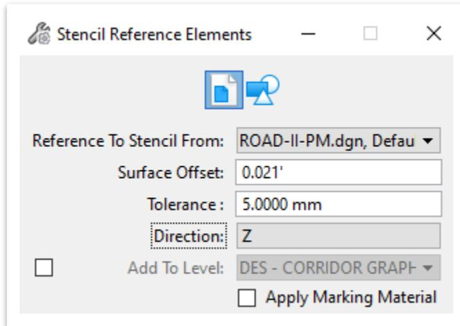
6. Notice the pavement markings now show up on the surface of the 3D model. Currently, Bentley has logged a defect where the surface offset is not applying. As a workaround, open the references for the **3D** model and change the stencil reference **Z** value to **0.1** to create an offset from the surface. **Note:** The construction display setting has been turned off in the screenshot below, which can be accessed in the **View Attributes** tool.
