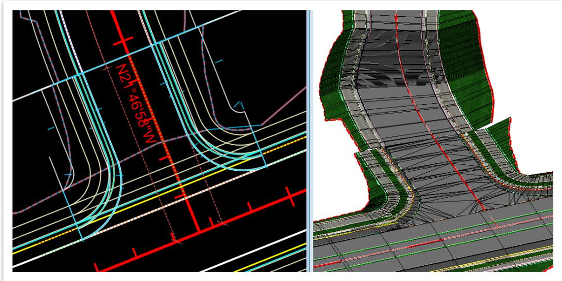
15. Notice that the civil cell automatically lined up with the mainline **PSHCG**, but it did not line up with the side road shoulder. To fix this, first locate the **SR PSH CTRL** line. The easiest way to find the line is to locate the area in the curb return where the line is hidden but is not underneath any other elements. Move the cursor to where the arrow is pointing in the screenshot below so that the line appears and then select the line.
