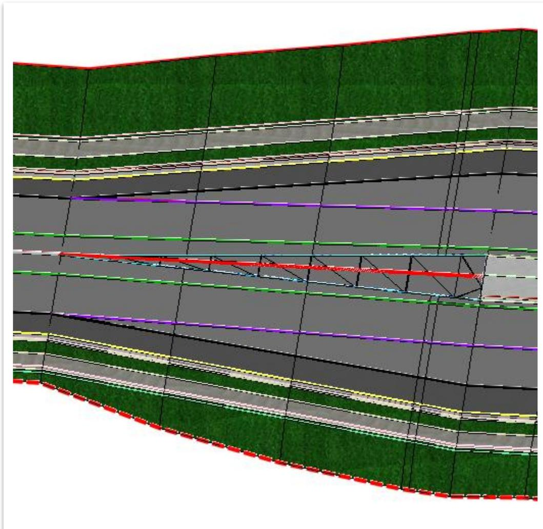
33. Next, select the **Curb - CTRL** feature definition (**Roadway >> Model Control - 2D Plan >> Curb and Gutter**).
