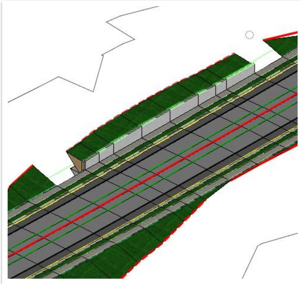
26. Notice that the corridor cannot transition between the cut of the end condition and the fill of the retaining wall before the next standard template drop. These conditions would have to be fixed using **Key Stations**. If this level of detail is not required in the 3D model, just update the plan view by drawing a line connecting the cut and fill lines using the **Prop End Condition - Fill Tie** feature definition (**Linear >> Roadway >> Grading and Ditches**).
