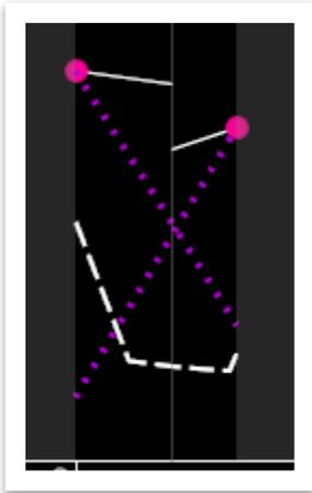
39. Now, draw two new lines that follow the first two lines drawn in the previous step, to create a **V ditch** and then complex the two lines and set the line to **active**. **Note:** The automatically drawn **3D** lines might still be in the 3D model. You can delete those lines now, if necessary.
