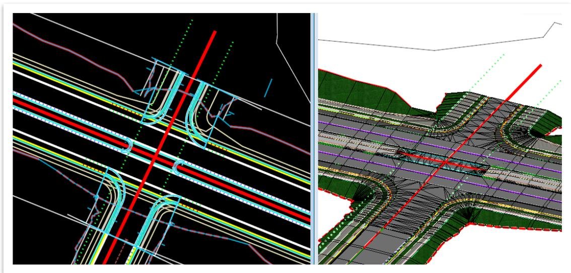
3. Select the **Ramp CL - CTRL** feature definition (**Linear >> Roadway >> Model Control - 2D Plan >> Sidewalk**) and set it to active.
