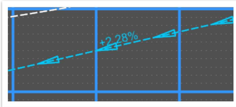
11. To add the **Begin/End** labels, open the **Civil Labeler** tool (**OpenRoads Modeling >> Drawing Production >> Labels**). Under the **TDOT - Design - Profile** folder, select the **Special Ditch Begin LT** and **Special Ditch End LT** labels. **Note:** Only the **End Ditch** label is shown below for reference. The special ditch is labeled in the direction of stationing, hence the End Special Ditch notation.
