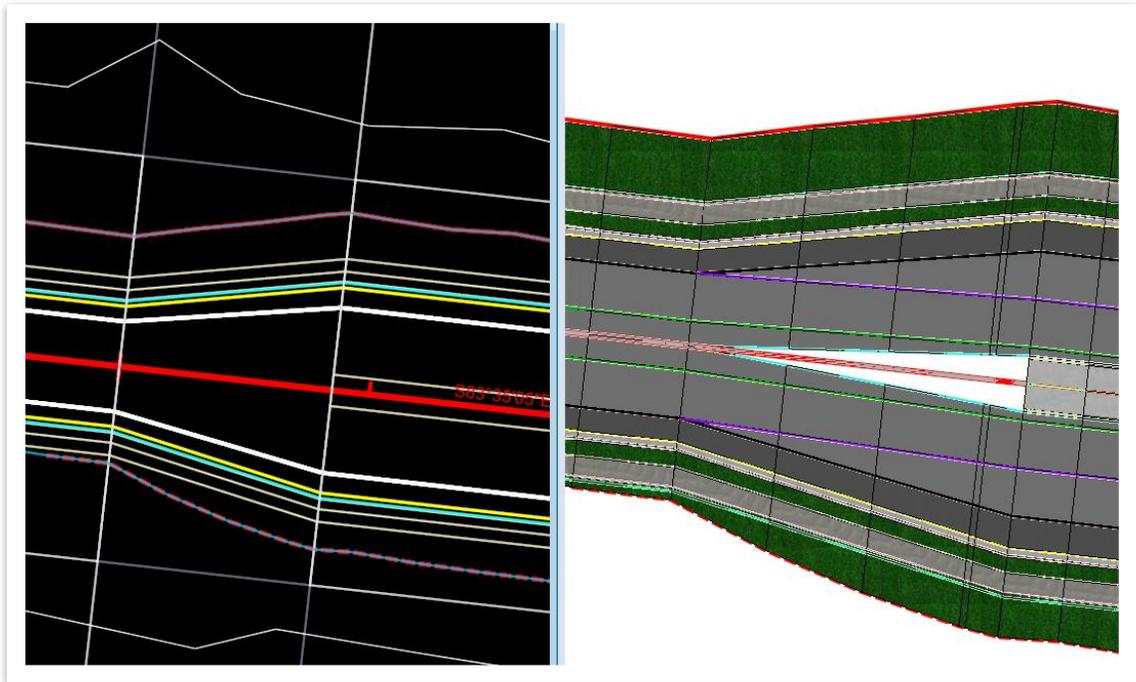
22. Next, we need to add a **surface** for the area that did not fill in from the transition and add a **median nose**. Select the **C&G Flowline - CTRL** feature definition (**Linear >> Roadway >> Model Control - 2D Plan >> Curb and Gutter**) and set it active. Make sure **Create 3D Automatically** is toggled on.
