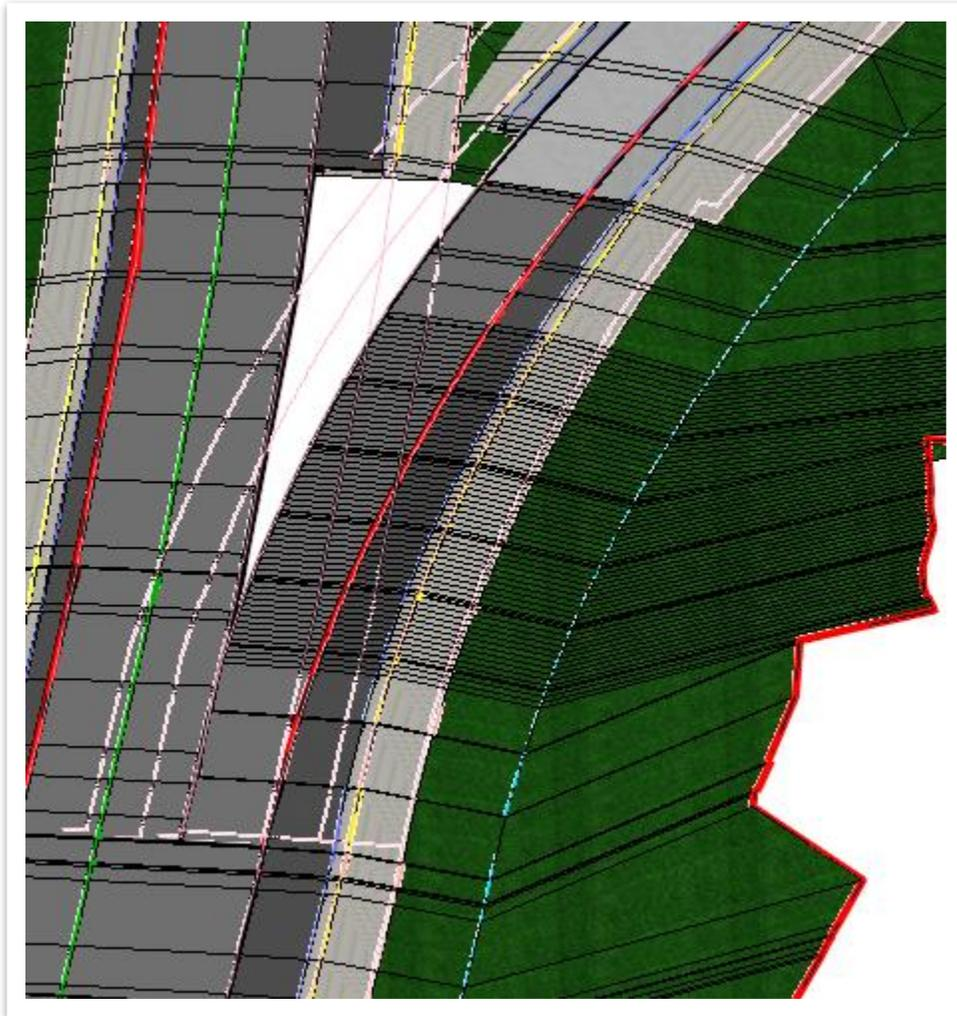
25. Next, we will model the gore between the templates. Go ahead and turn off the **ROAD-II-RG-Proposed.dgn** reference file.
