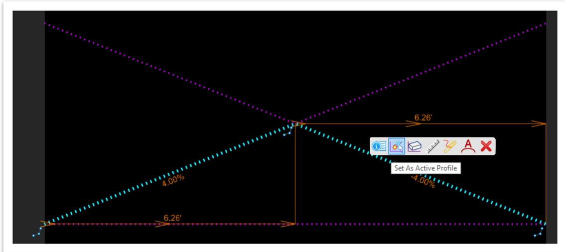
40. Now, we will create another terrain. Open the **Create Terrain Model From Elements** tool (**OpenRoads Modeling >> Terrain >> Create**). Turn off the **DES - CORRIDOR GRAPHICS - Design** and **DES - MODEL - Lines - Curb Flowline** levels to make it easier to select the two lines. Select the **Curb** line with the new profile and then select the **CR\_BACK\_TOP\_RM** line.
