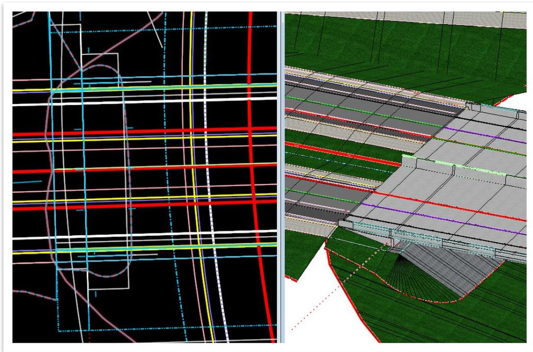
15. Now, a **parametric constraint** needs to be added on the **PSH\_R** side of the abutment to tie the I65 slope to the abutment slope. Open the **Create Parametric Constraint** tool (**OpenRoads Modeling >> Corridors >> Edit >> Edits**). Select the **Abutment Tie In Right** corridor.
