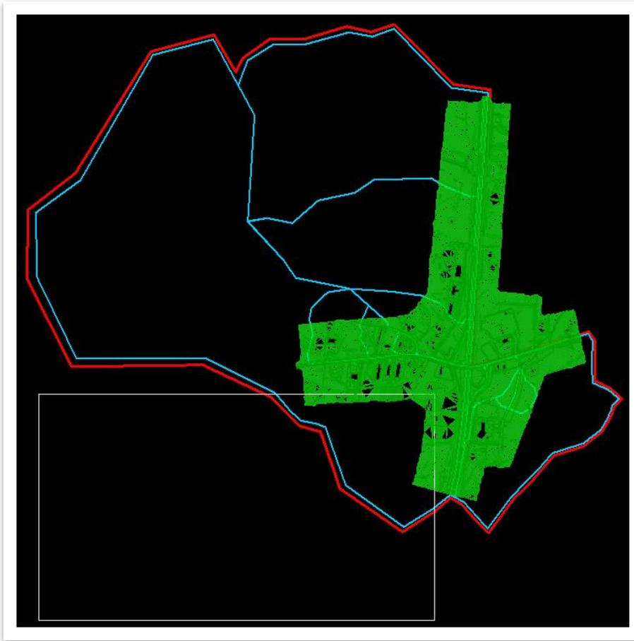
13. Now, we will go through the steps to create a clipped terrain model from the **1688469NE** tile. Open the **Create Clipped Terrain Model** tool (**OpenRoads Modeling >> Terrain >> Create >> Additional Methods**).
