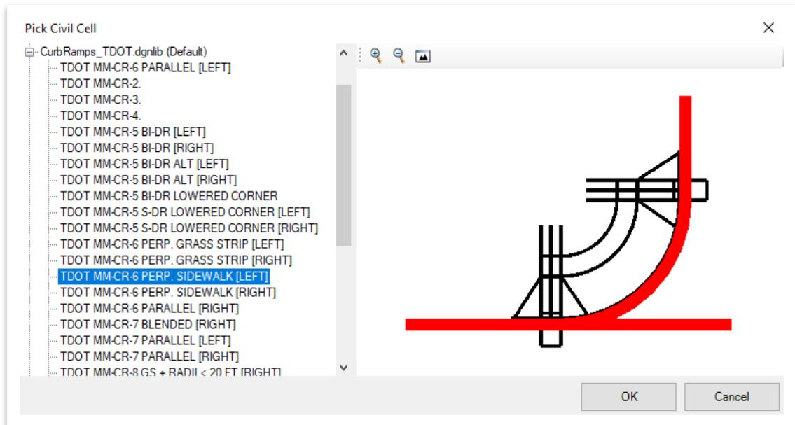
14. Select the following reference lines in order: the intersection (curb return) **CR Flowline (1)**, the intersection (curb return) **CR Back Top (2)**, the mainline **CR Flowline (3)**, and the mainline **CR Back Top (4)**.
