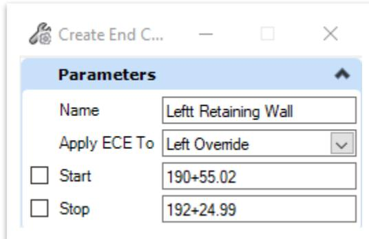
18. The **Left Override** window should open. **Right** click in space and select **Delete Components**. Draw through the **EC\_FILL\_TIE\_L** line and click **OK**.
