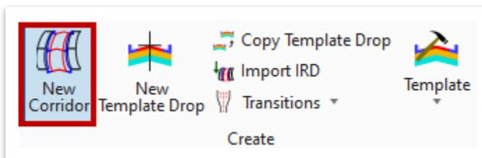
5. Select the **EX CL** alignment as the **Corridor Baseline**. **Right** click to select the active profile of the **EX CL**, which is the existing terrain. Then, change the **Name** of the corridor to **Unsuitable Material**.
