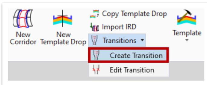
3. Select the two template drops in the **2D** plan view. The **2D** and **3D** model will both render a **transition**, but only for the **EOP** and the **paved shoulder**.
