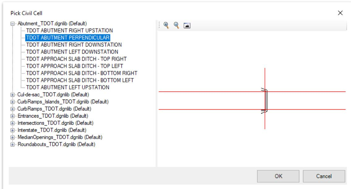
7. In the **2D** view, follow the prompts and select the **Abutment CTRL (1)**, **PSH\_L (2)** and the **PSH\_R (3)**. **Note:** This cell works in both left and right directions. The selection order for the other side abutment placement would be the **PSH\_R** line and then the **PSH\_L** line.
