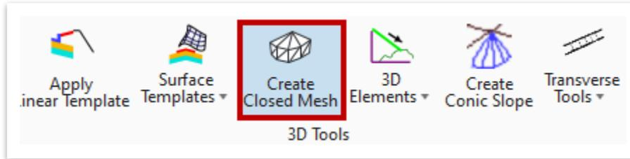
17. Within the **Create Closed Mesh** dialog box, select the following settings. **Note:** The depth should be project specific so ensure that the depth is deep enough encompass all cut needed for a project. Since we do not have a lot of major cut areas in this example, it does not have a large depth.
