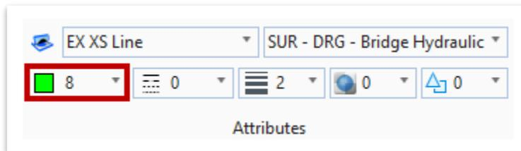
21. Open the **Place SmartLine** tool once again (**OpenRoads Modeling >> Drawing >> Placement**) and select the settings shown below.
