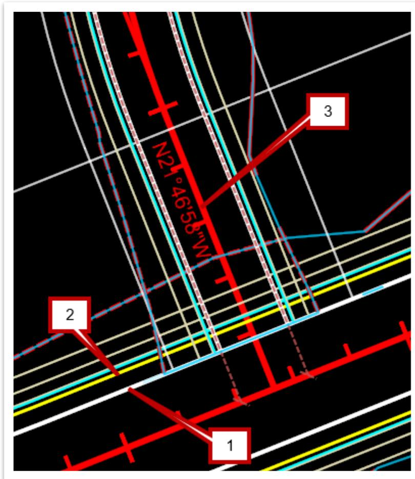
4. Make sure the placement looks correct by clicking on the **control lines**. In this exercise, there should be no need to reverse the direction of the reference lines. **Right** click to accept line directions. Next, select the Side Road corridor to clip and then **right** click to accept. Lastly, **left** click to accept the civil cell placement.
