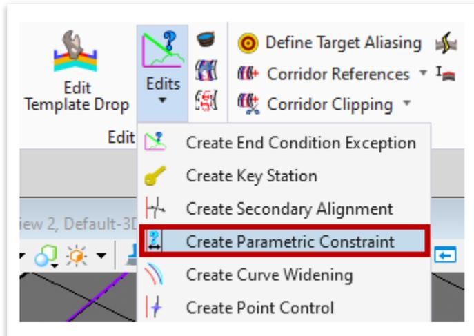
17. Select the **start** location (Station **83+49.39**) and the **stop** location (Station **85+25.65**). Within the **Create Parametric Constraint** dialog box, change the **Constraint Label** to **GSH\_L Width** and the **Start Value** to **-10.0**. Left click through the prompts to accept.
