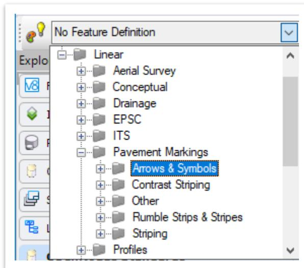
**Arrows & Symbols:** Contains arrow and symbol line styles that are setup to be placed at set distances defined by TDOT standard drawings.
