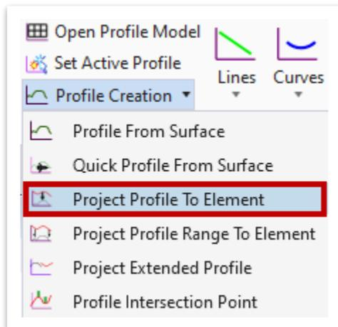
4. Select the **special ditch** centerline in **plan** view (Station **152+50.00** to Station **162+50.00**) and then select the **mainline** centerline. Open the roadway **profile** view, if not already open, and you should now see the **special ditch** profile projected onto the roadway profile.
