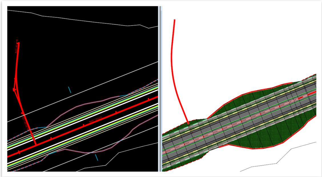
2. Select the **Retaining Wall - CTRL** feature definition (**Linear >> Roadway >> Model Control - 2D Plan >> Barrier**).
