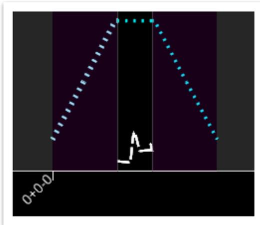
34. Now, open the **Create End Condition Exception** tool (**OpenRoads Modeling >> Corridors >> Edit >> Edits**) and select the **I65** corridor. Name it **Box Culvert Left** and set the **Apply ECE To** option to **Left Override**. **Note:** When setting the **Start** and **Stop** stations, do so right at the start and end of the wingwalls but **do not snap** to the wingwalls. Your stations may vary depending on where you clicked.
