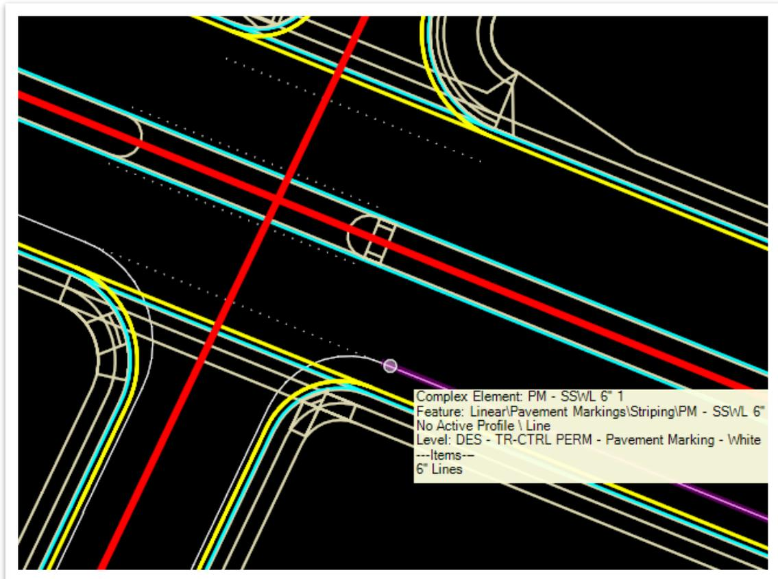
11. Go ahead and turn the **DES - Model - Lines - Pavement Edge** level back on. We are going to place the inside yellow lines along the eastbound lanes of the mainline corridor. First, locate the **5-lane** section of the main corridor at the beginning of the stationing. The first section of striping will be without the bi-directional markers. Select the **PM - DBYL 6" [RIGHT]** feature definition (**Linear >> Pavement Markings >> Striping**).
