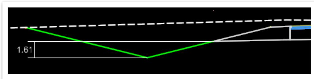
14. Now, switch back to the **Drainage and Utilities** workflow. Open the **Place Conduit** tool (**Drainage and Utilities >> Layout >> Layout**). Select the **V Ditch - User Input** feature definition (**Conduit >> StormWater >> Ditches >> Standard V Ditches**) and leave the **Description** as **No Description Selected**.
