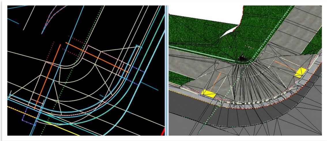
16. Zoom in and notice that the sidewalks have been tapered and adjusted to meet the back of the civil cell ramps. This is because the civil cell is built with the maximum slope of **8.33%** and the sidewalk needs to be widened to match the civil cell max slope. **Note:** For all civil cells that have two ramps that wrap around the radius, the civil cell will not work well if the ramps are two different slopes.
