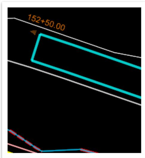
3. Next, open the **Edit End Condition Exception** view. This can be done in various ways: by hovering over the end condition exception in **2D** view, by **right** clicking on the end condition exception in the **Properties** view, or by navigating to the end condition exception section in the **Corridor Objects** tool.
