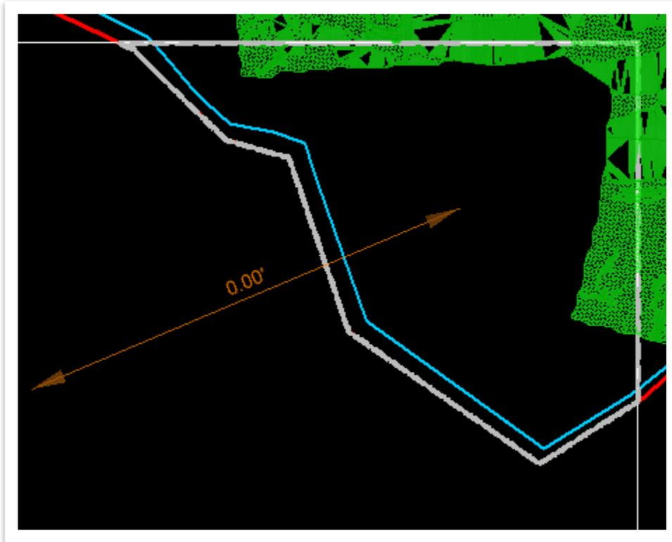
17. If you have the surveyed triangles turned on, go ahead and turn off the **SUR - DTM - Triangles** level within the **ROAD-II-ET-Terrain.dgn** reference file. Now, select the clipped terrain and turn on the **Major Contours**. Once reviewed, turn them back off so that the file processing is more efficient.
