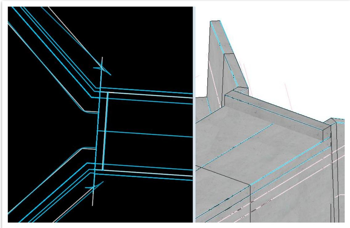
29. The box culvert model is now complete. The last item we need to do is target the **slope lines** to the new box culvert model. Go ahead and open the roadway corridor file (**ROAD-II-BC-I65 Corridor.dgn**) and attach the **ROAD-II-BC-Drainage Structures.dgn** file that was just created. Within the drainage structures file, turn off the **DES - CORRIDOR GRAPHICS - Design** level.
