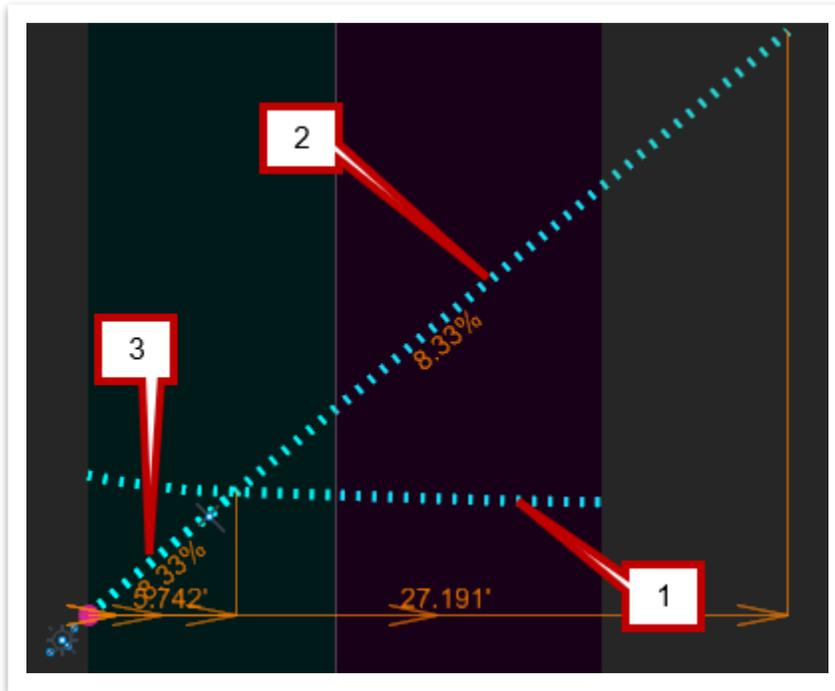
12. Go ahead and change the slope of **line 2** to **6%**, which will update the slope of the right ramp, and then turn all levels back on.
