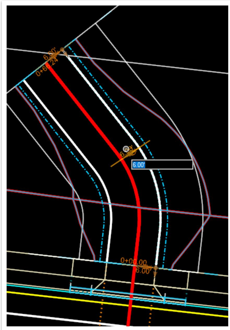
24. The corridor now needs to be adjusted to make sure the driveway cross slopes mirror the profile grade of the mainline corridor. Open the **DR EOP L CTRL1** profile. **Note:** This is only done so that the model aligns. A PDF set of plans will not show this level of detail.
