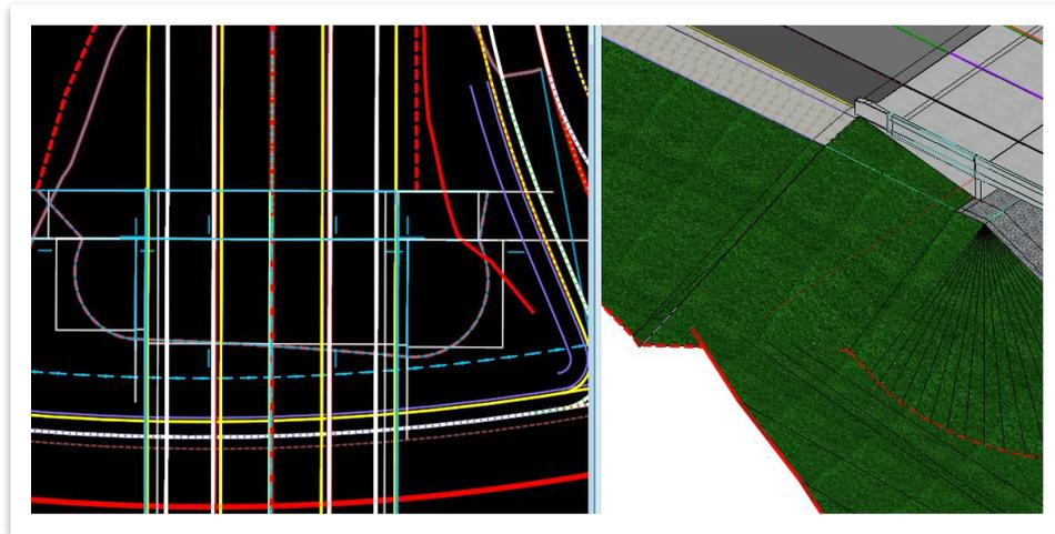
17. Repeat the previous step and create a **parametric constraint** on the **PSH\_L** side of the abutment. Set the **Start Value** to **50.00%** and the **Stop Value** to **33.33%**.
