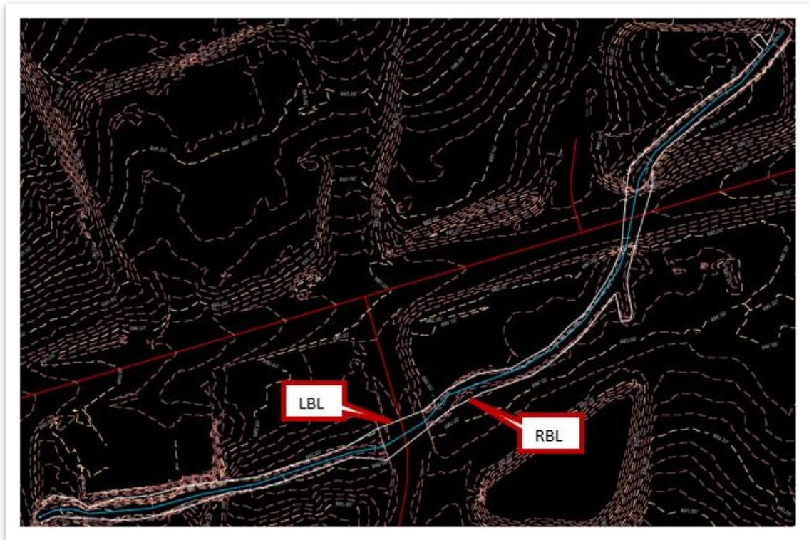
16. Next, we need to draw in the left overbank line (**LOB**) and right overbank line (**ROB**) using a **35'** offset from the LBL and RBL. Turn the **ROAD-II-HEC-Survey.dgn** reference file back on. Using the same **EX Bank Line - Top** element template, change the line color to **11** (purple). **Note:** The user can select any line style attributes. For this exercise, however, a specific color was chosen to provide a visual difference between the features drawn.
