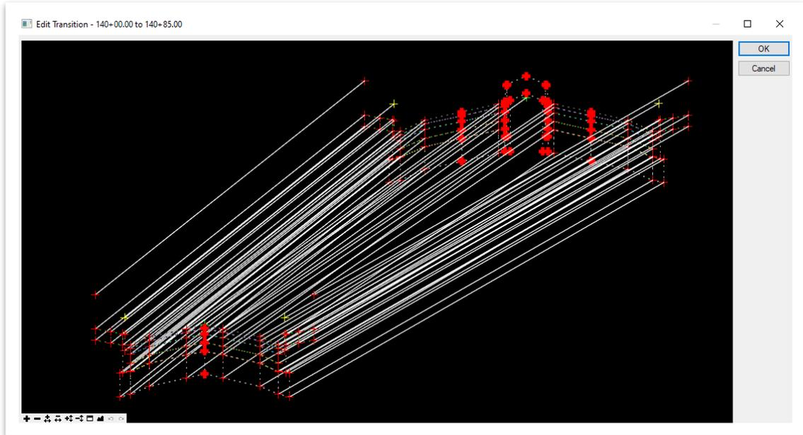
6. **Right** click on one of the template ends and notice a **Move Template** prompt appears. This allows the selected template to be moved around within the window to see a better view of what is linking.
