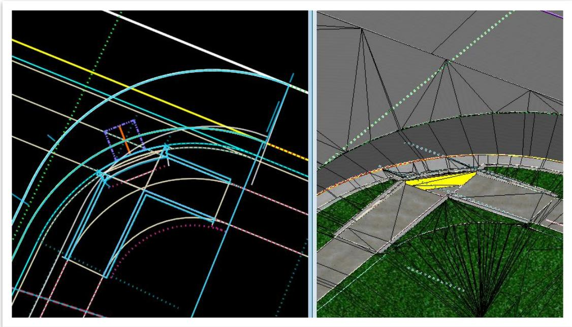
28. Next, locate the east median opening between the two **CR-7** curb ramps placed earlier in the exercise. With the **Ramp CL - CTRL** feature definition (**Linear >> Roadway >> Model Control - 2D Plan >> Sidewalk**) still active, draw a geometry line **6 feet** off the back of the median opening nose, perpendicular to the **EOP** lines.
