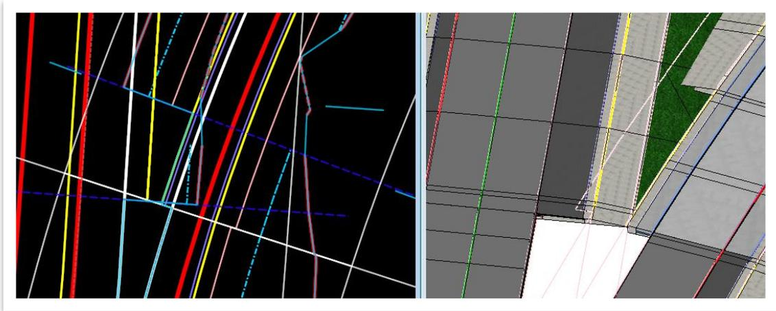
28. Once completed, open back up the **ROAD-II-RG-I65 Corridor.dgn** file. Confirm that the **ROAD-II-RG-Proposed.dgn** reference file is turned off. It will not be needed for the remainder of the modeling.
