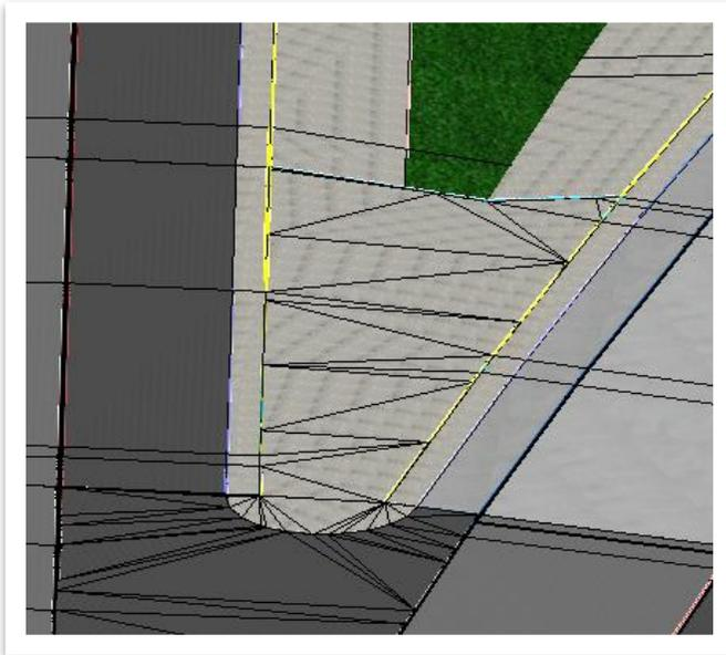
54. Lastly, we need to add the break line down the middle of the surface. Right click on the **Gore Aggregate** terrain once again in the **Explorer** and select **Add Feature**. Select the center ditch line drawn and then right click to accept. Set the **Feature Type** to **Break Line** and then click through the remaining prompts to accept. Notice that the ditch has been added to the surface and the modeling of the ramp gore is complete.
