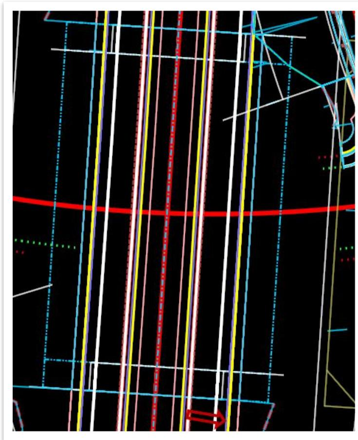
28. Click through the prompts, and then data point with the intersection snap to place the point at the intersection of the **PSH\_R** and the end of the concrete barrier.
