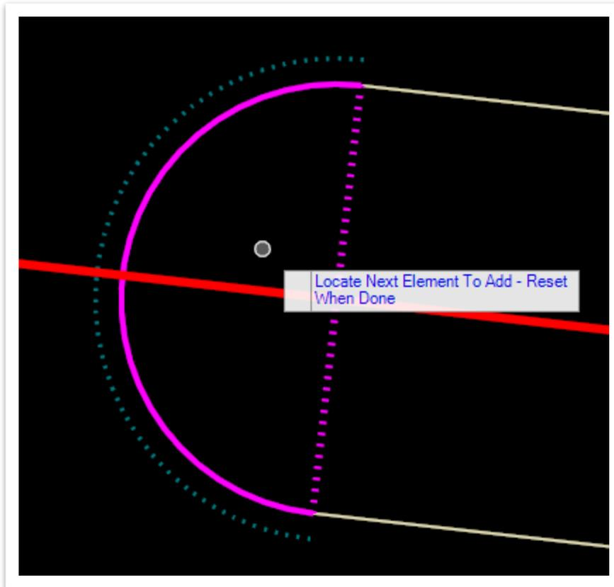
45. **Right** click to accept those two lines, and then make sure the **Feature Type** is set to **Break Line**, the **Edge Method** is set to **None**, and the **Feature Definition** is a **Civil Cell**. Name the terrain **Median Nose**. **Left** click through the prompts to accept.
