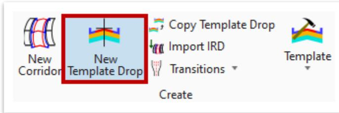
19. Select the **TS-4 RIGHT (1LN) - 4 LAYER** template (**Linear Templates >> TDOT Typical Sections >> Undivided**). Then, select the **ramp** corridor and place the template from the start of the ramp alignment (Station **500+00**) to where the concrete ramp begins (Station **502+51.09**).
