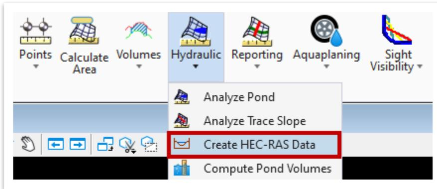
27. Notice the first prompt: **Locate First Section Line**. Select the **first** cross section line on the **downstream** end of Pumpkin Creek (north side of the roadway). Then, select the remainder of the cross section lines in the **upstream** direction and **right** click to end the selection.
