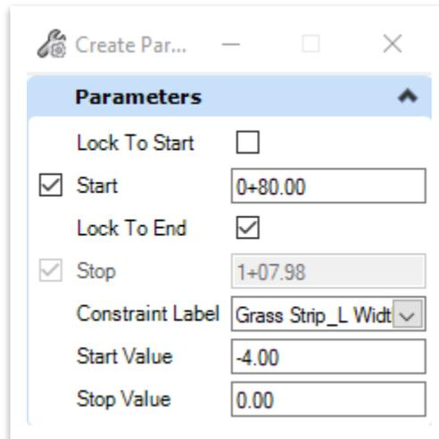
19. Repeat the previous step for the right grass strip (**Grass Strip\_L Width**) by selecting the right intersection civil cell linear template. The start station will be **0+92.00**. Notice the updates once the **Parametric Constraint** has been added. **Note:** Since the civil cell has two identical template drops on each **PSH CTRL** line, the line and parametric constraint names are the same (i.e., the grass strip name is the same for the right side template drop).
