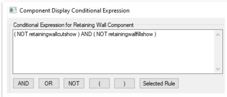
21. Click **OK** to close the **Component Display Conditional Expression** tool, and then click **Apply** and **Close** to close the **Component Properties** window. Test the file and the retaining wall should only show up when the cut line is more than 12 feet horizontal, and it should not show up when in fill.
