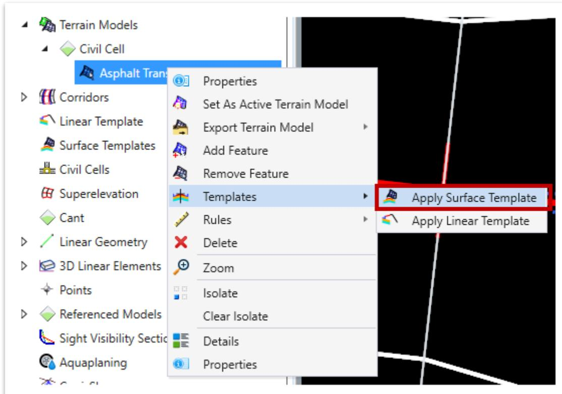
31. Select the **SURFACE - 4 LAYER** template (**Linear Templates >> Civil Cells >> Surface**) and left click through the prompts to accept.
