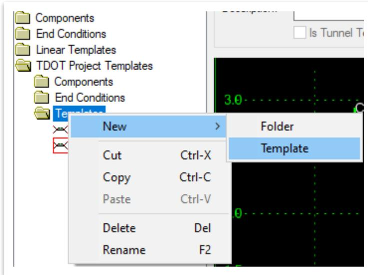
6. An empty template should now appear. Scroll up and select the **TS-5B (6LN) Approach Slab** template (**Linear Templates >> TDOT Typical Sections >> Bridge >> Approach Slab**). Click on the template once so that the preview shows up in the bottom left corner.
