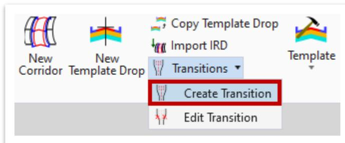
Transitions work by targeting points of the same name between the two template drops selected. The template will automatically connect points of the same name when a new transition is created. However, the transition will need to be edited due to one of the two reasons listed below:
