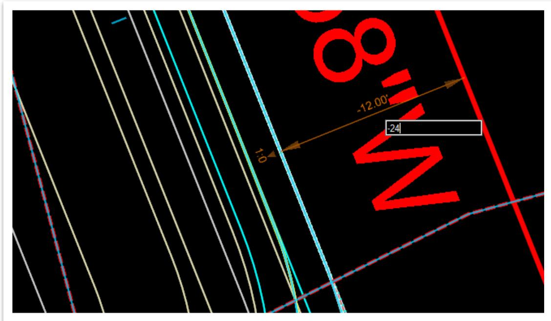
9. Now, we will use a **point control** to add a turning lane to the side road corridor. Select the **Prop EOP - CTRL** feature definition (**Linear >> Roadway >> Model Control - 2D Plan >> EOP**) and set the feature to active.
