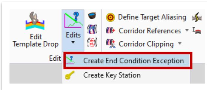
8. Select the mainline corridor and then select **Right Override** for where to apply the **End Condition Exception (ECE)** to. Set the start and stop locations around the start and end of the retaining wall. Try to get as close as possible but do not snap to the line created.
