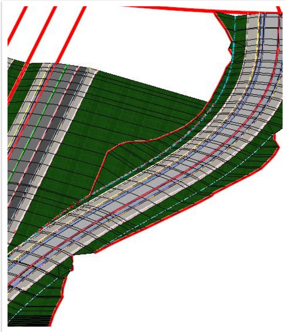
14. Open back up the **ROAD-II-RG-Ramp Corridor.dgn** file and then open the **Add Corridor Reference** tool (**OpenRoads Modeling >> Corridors >> Miscellaneous >> Corridor References**). Add the **ditch** line as a corridor reference to the ramp corridor by selecting the ramp corridor and then the ditch line created.
