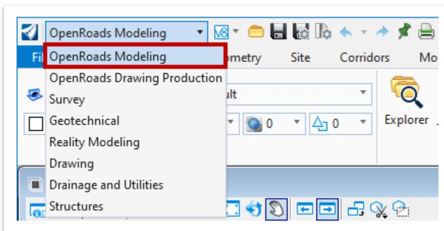
11. Now that the OpenRoads Modeling workflow is active, we will setup the recommended TDOT user interface which will ultimately assist in more efficient modeling efforts throughout this manual. Make sure the **Explorer tool (Open Roads Modeling >> Home >> Primary)** is docked/pinned on the left side of the screen. **Note:** It should automatically default to this location once opened.
