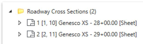
35. Since cross section sheets are located after the proposed profile sheets, we must edit the **Start Number** in the **Sheet Numbering Controls** for the **Roadway Cross Sections** folder. By default, the start number is set to **1**. For this exercise, we will assume that the roadway cross sections start at **22**. Go ahead and highlight the **Roadway Cross Sections (2)** folder.
