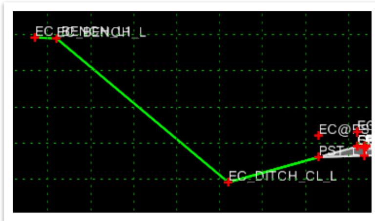
16. Next, double click on the **EC\_Bench\_L1** point to open the **Point Properties** dialog box. Deselect **End Condition is Infinite**. Then, click **Apply** and **Close**.
