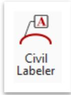
The Civil Labeler is a new tool in OpenRoads Designer 10.10 Connect Edition. The Civil Labeler tool will eventually replace the place label tool. The TDOT Civil Labeler tool is built to replace the labels created for the Place Label tool on a 1 to 1 basis with additional labels created for the enhanced capabilities of the Civil Labeler tool.
