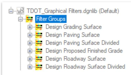
Once a graphical filter group has been selected from the **TDOT\_Graphical Filters.dgnlib** (default) through the **From Graphical Filter** tool (**Terrain >> Create**), this group and its filters will be displayed under the active design file and can be edited.
