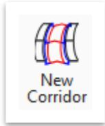
This tool is the first step in corridor design, and it allows the user to identify the controlling alignment, set the feature definition and name the corridor. Once the corridor has been created, the software automatically advances to the **New Template Drop** tool.
