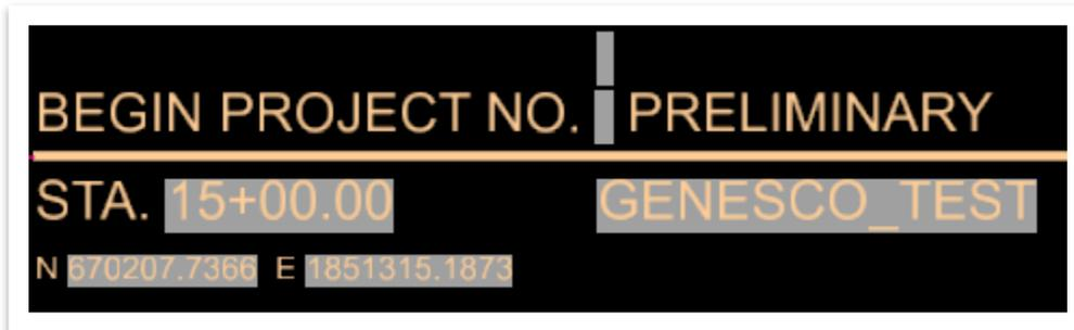
39. Repeat steps **31-38** to place the **End Preliminary** label. This time select the Element Template: **End Project Preliminary** and when placing the label, select **Cell Name:** `_DES - TS - PROJ DESCR - End - PRELIM - Proj Less Than 2 Miles`. Snap to the **lower** blue dot above the Special Notes.
