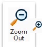
These tools allow the user to zoom in and out of the drawing at a defined **Zoom Ratio**. Zoom Out zooms from the center of the window and Zoom In creates a rectangular overlay showing the new window area.
