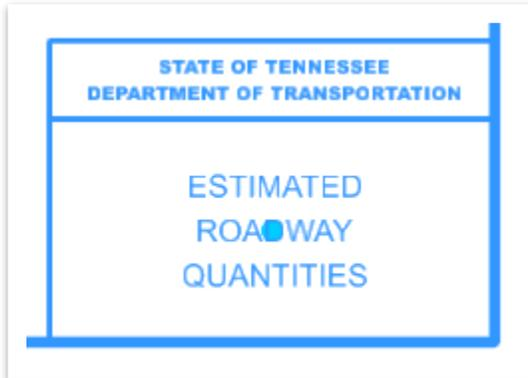
11. Before the actual Estimated Roadway Quantities excel document is placed in the dgn file, let's select the applicable Element Template. Go to **Drawing >> Home >> Attributes** and select the Element Template drop-down menu. Then, select the **Roadway - Text** element template (**Design >> Annotation >> Plan Sheets >> Proposed**). **Note:** If you forget to set the element template, the excel data will come in on the **Default** level and not print based on the setup of the TDOT print style.
