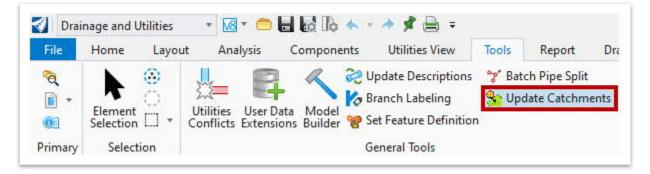
In addition, the user can now apportion catchment runoff to gutters that flow to a sump inlet. If a catchment is connected to a sump inlet, which has two gutters connected to it, then the flow from the catchment should be apportioned between the gutters, as opposed to the same flow being assigned to both gutters.
