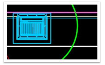
21. For clarity, let's view the model in **2D**. Within the **References** window, turn off the **Bowling\_Drainage.dgn** file (**Model: Default-3D**). The catch basin should now only have the 2D linework displayed.
