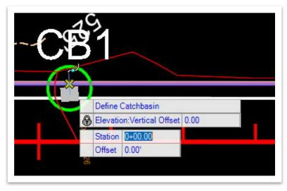
14. Move the cursor towards the location of CB1. Press the letter O on the keyboard. Notice the cursor prompt: Select a reference element or Reset to return to command. Note: If ever the Sta/Off functionality does not seem to work, you will likely need to re-select the reference element in which to base the Sta/Off by doing this step again.
