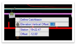
17. Move the cursor towards the location of **CB1**. Hit **TAB** once again to edit the station and offset. Key-in station **19+08.50** and offset **-15.90**' for this exercise. Hit the **TAB** or **Enter** key after each entry so that it locks in place. Left click to accept.
