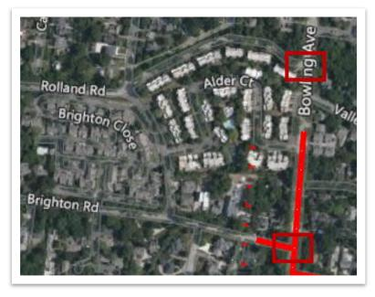
Since there is not any geometry linework at the Rolland Rd intersection, we need to draw a line so we can snap to the location easier. Open the Place Smart Line tool (Drainage and Utilities >> Drawing >> Placement) and draw a line like what is shown below.
