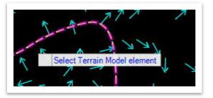
4. Notice the cursor prompt: Select Start Point for Trace Path. Select any point as the Start point. This results in a flow path shown from the cursor to the furthest point that the water drop reaches. This tool helps in analyzing flow patterns for a project. Note: The data shown in the screenshot will vary depending on what start point you selected.
