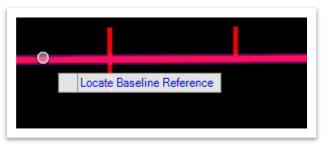
8. Next, you will be prompt to select the Rotation Mode. Left click to accept and a new prompt will appear asking you to Locate Reference Element for Rotation. Select the Bowling centerline and hit Enter. Left click to accept the rotation. Alternatively, you could select the Rotation Mode in the Place Node dialog box. In this exercise, key-in a rotation angle of S43^05'12.8"E. Left click to accept and then hit ESC to clear the tool.
