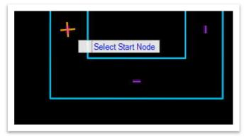
4. A white conduit line should now appear with the end attached to the cursor. Notice the cursor prompt: Select next node to make a connection. Move down to CB3 and select the far right connection point, highlighted in red. Left click to accept placement of the conduit and then right click to clear the tool.
