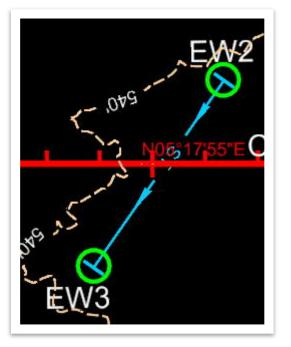
9. Confirm that the two new endwalls (EW2 and EW3) and the new conduit (CrossDrain RCP) have been added to the Drainage and Utilities model within the Explorer. Note: As a reminder, if the conduit does not show, click the Refresh icon under the Drainage and Utilities Model header. If the conduit still does not show, close and re-open the Explorer.
