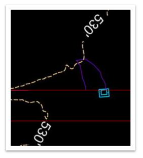
5. Place a <u>second</u> catch basin within the delineated area of the first catch basin using the same structure type and catchment.
