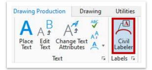
Within the civil labeler window, select the Conduit Size label (TDOT Civil Labeler >> TDOT - Drainage and Utilities - Plan >> Proposed). Change the Leader to None and the Rotation to View Horizontal. Leave all other predefined TDOT settings as-is. Click Place.
