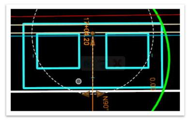
27. Click the orange station text and key-in **17+04.25** and then hit **Enter**. Notice that the structure location automatically updates to the precise sag location along the roadway.
