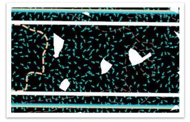
4. The Analyze Pond dialog box should open. Hover over the different pond areas and you will notice that the pond data will populate. Within the dialog box, select the Prop Pond - Top feature definition (Linear >> Roadway >> Pond) and then left click on the shape as shown below. This will add the pond area to the model. Note: Units for Volume and Area are cubic feet and square feet respectively.
