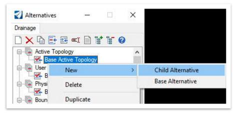
3. To keep all alternatives, the user should create a child alternative with a unique name and then link the respective topologies to the scenarios. This will run the scenarios only on those elements, which will minimize the need to check / uncheck the topology each time. If running an analyze scenario, select the analyze scenario and link the desired topology that you want to run on it.
