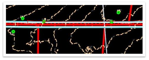
3. We will now place catch basins at the approximate locations shown. The location of CB3 is a sag point on the roadway. Before we place any catch basins, it is recommended to review the centerline profile. Select the <u>Bowling centerline</u> and open the Open Profile Model tool. It can either be accessed within the heads-up display (2<sup>nd</sup> icon) or within the ribbon under Drainage and Utilities >> Utilities View >> Drawing Views.
