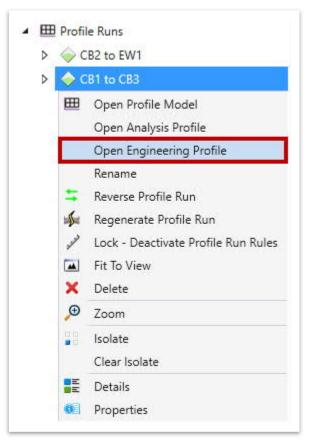
11. In the Engineering Profile window, review the Nodes, Conduit, Ground Elevations, Inverts, etc. to verify if the inlets and pipe are connected correctly in the direction of flow, along the storm drain. Note: You may review the engineering profile of the other profile run (CB2 to EW1) in the same manner.
