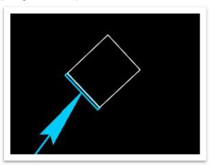
Now, select the Rip Rap (Proposed) element template (Design >> Area Patterns >> Roadway) so that the riprap will be placed with the correct symbology.
