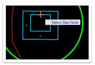
Notice the next cursor prompt: Select next node to make a connection. For CB3, snap to the top connection point as shown below. The green gutter should now be placed between CB1 and CB3. Bypass flow will go to CB3.
