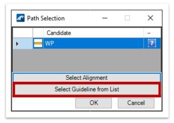
17. Another **Path Selection** dialog box should open. Select **P\_1** as the **Guideline Point Name**, which corresponds with the top right edge of the approach slab. You can zoom in and out of the graphical display of the selected template to confirm which point name corresponds to which point on the template. Click **OK**.
