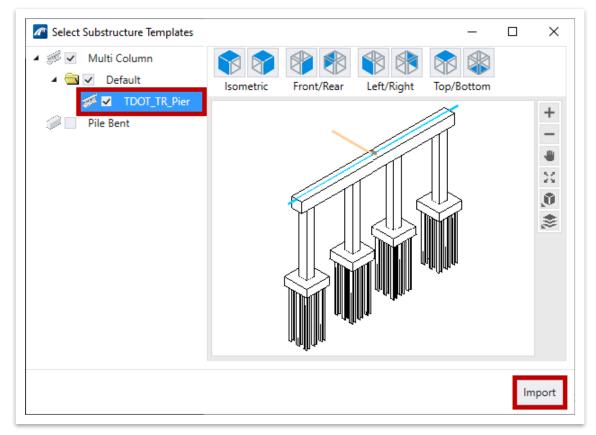
4. To begin pier placement, open the **Place Pier** tool (**OpenBridge Modeler** >> **Home** >> **Substructure**).
