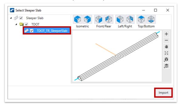
4. To begin sleeper slab placement, open the **Place Sleeper Slab** tool (**OpenBridge Modeler >> Home >> Approach Slab**).
