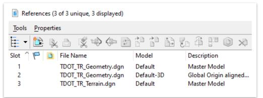
6. Select the **Fit View** button at the top of the view windows for both **View 1 - Top** and **View 2 - Isometric**. The newly referenced files will now be visible.
