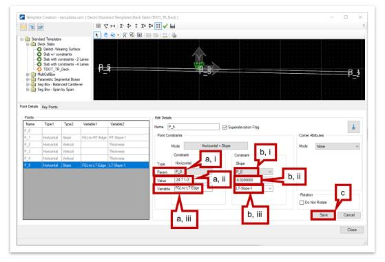
9. Click **Close** to close the **Template Creation** window. The new deck template is now complete and is ready to be used with the **Place Deck** tool.
