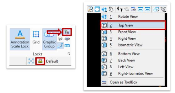
11. View 1 of the alignment should now be parallel with the screen. Go to File >> Save Settings or [Hold Ctrl] + [type] F to ensure the ACS rotation is saved.
