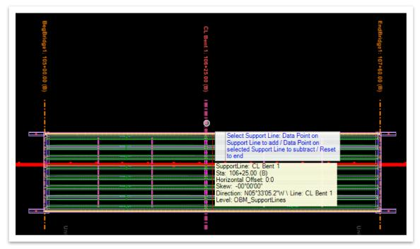
7. **Reset** (right click) in space to end placement. You can place multiple piers at once if needed prior to ending placement. **Data Point** (left click) to continue and confirm entries in the **Place Pier** dialog box.
