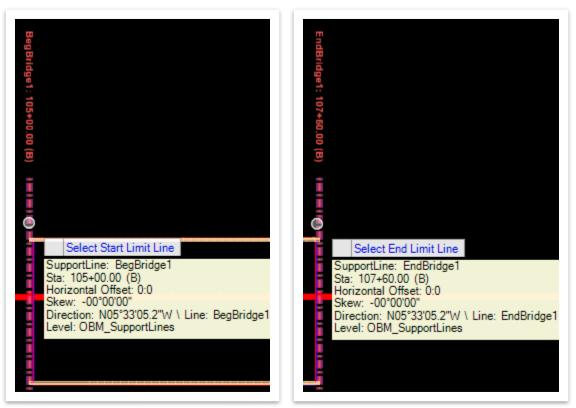
3. **Data Point** (left click) to accept the Limit Lines and then open the **Beam Layout** window.
