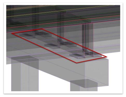
Now we will place the bearing lines at the abutments. We will place these bearing lines at the same time since the program knows which end bent is begin and which is end. Open the Place Bearing tool once again (OpenBridge Modeler >> Home >> Substructure).
