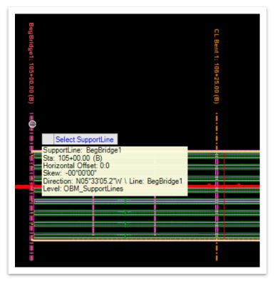
7. **Data Point** (left click) in space to confirm placement. **Reset** (right click) to close the **Place Abutment** dialog box and notice that the begin bridge abutment is now visible in both views.
