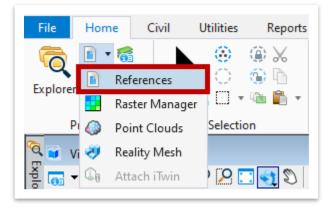
Click the Attach Reference button and browse to the TDOT\_TR\_Geometry.dgn file located here: C:\ProgramData\Bentley\OpenBridge Designer CE 10.10.20\ OpenBridgeModeler\Configuration\WorkSpaces\TDOT\_Standards\WorkSet s\123456.00\_OBM\_TR\dgn\. It should open to this folder by default. After selecting the dgn, click Open. Click OK in the pop-up alert about the file not belonging to the active workset.
