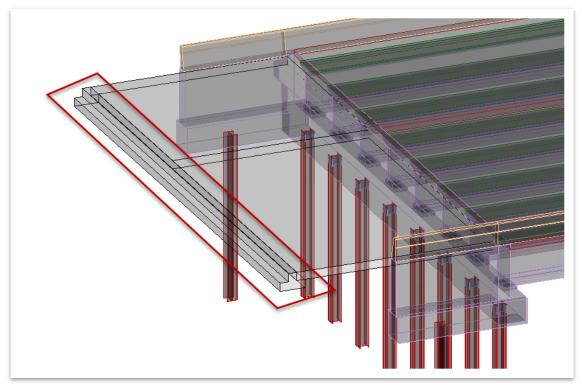
7. The full bridge model is now complete and can be referenced in the overall roadway model to complete the corridor. The model can now be used for a variety of advanced features, including quantity reports, elevation reports, clash detection, dynamic plans production, rebar modeling, digital twin asset management and more!
