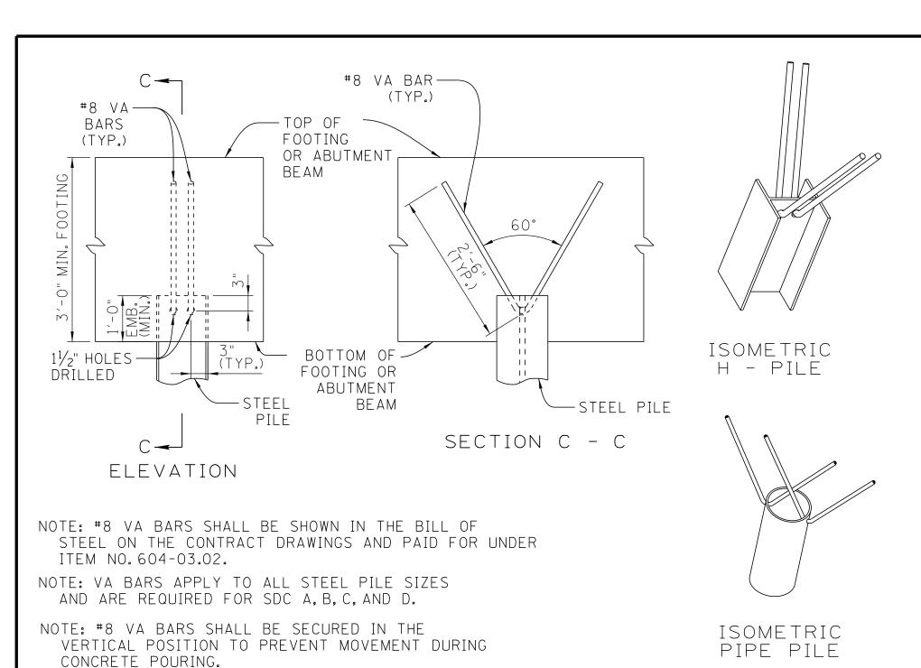
STEEL PILE SEISMIC ATTACHMENT DETAILS
