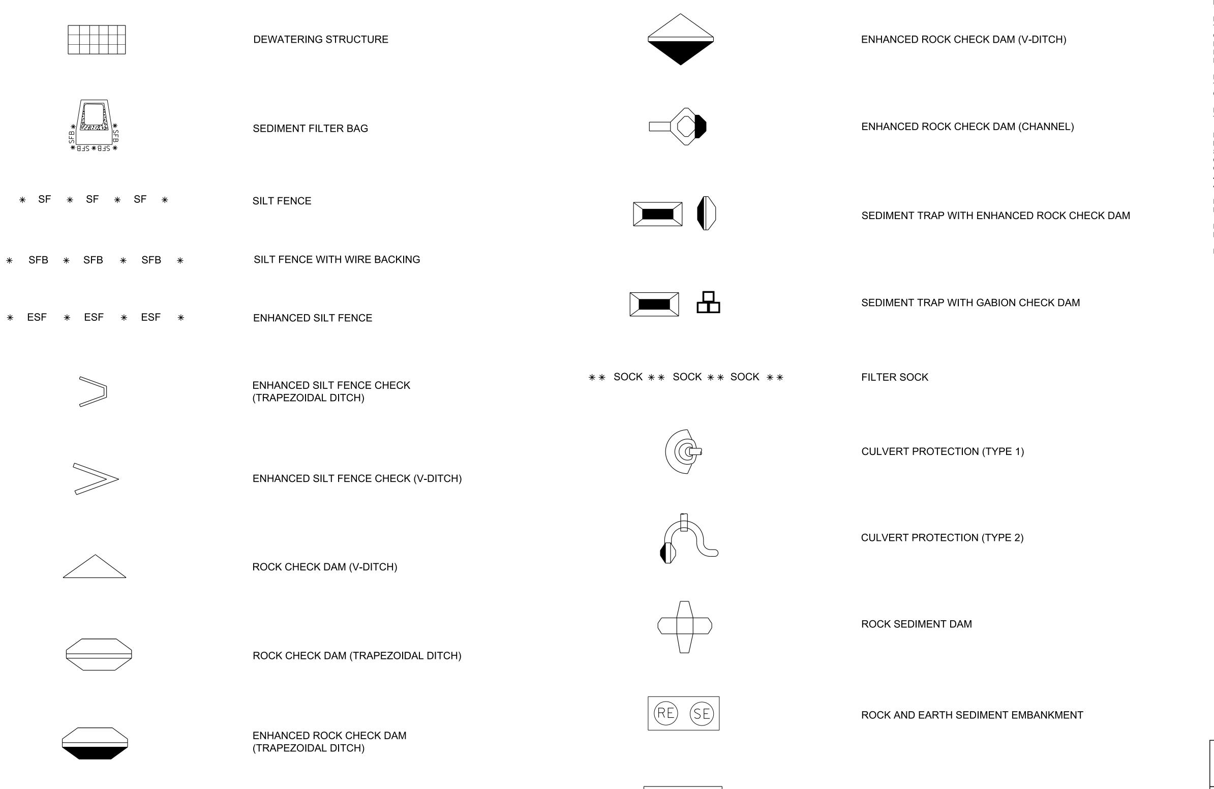
SEDIMENT CONTROL LEGENDS FROM OLD STANDARD DRAWING NO. RD-L-2 AND THE ESC-STR SERIES OF DETAIL SHEETS.
