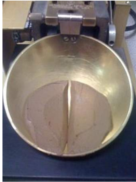
Figure 3.7: Atterbeg Test of Subgrade Soil
