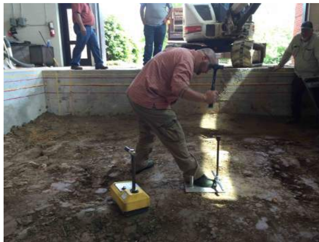
Figure 4.9: Test of Density and Compaction Degree of Subgrade Soil Using Nuclear Gauge
