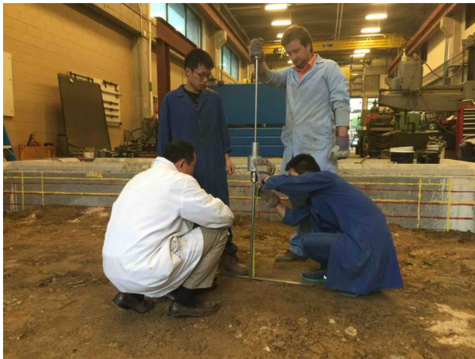
Figure 4.11: Dynamic Cone Test for Bearing Capacity of Subgrade
