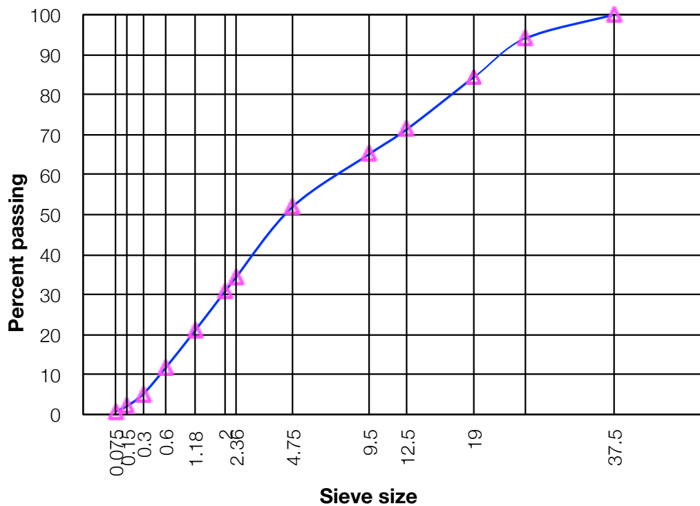
Figure 3.9: Gradation of Subgrade Soil Used in Test Pit
