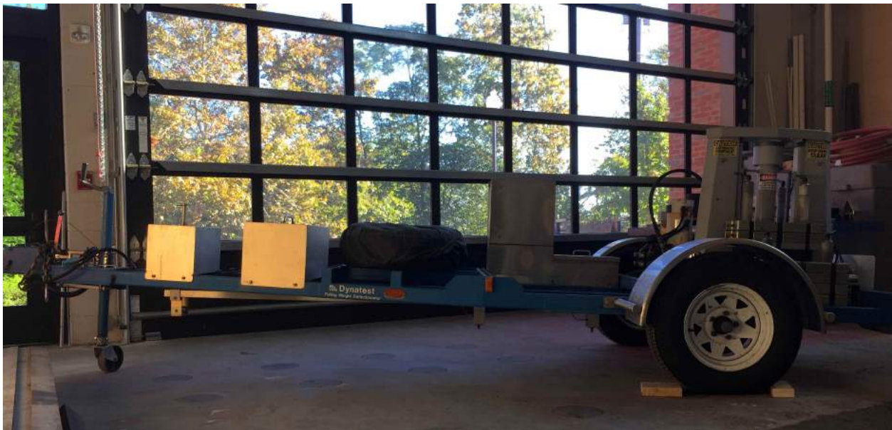
Figure 4.34: Falling Weight Deflectometer (model#: 8002-200)
