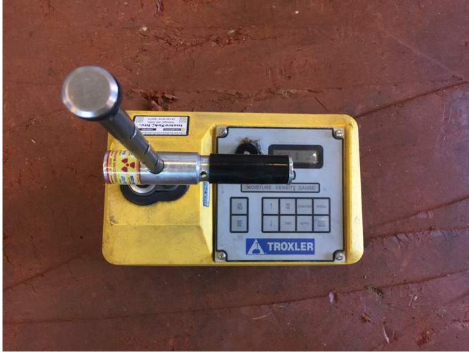
Figure 5.6: Checking Subgrade Density with a Nuclear Gauge
