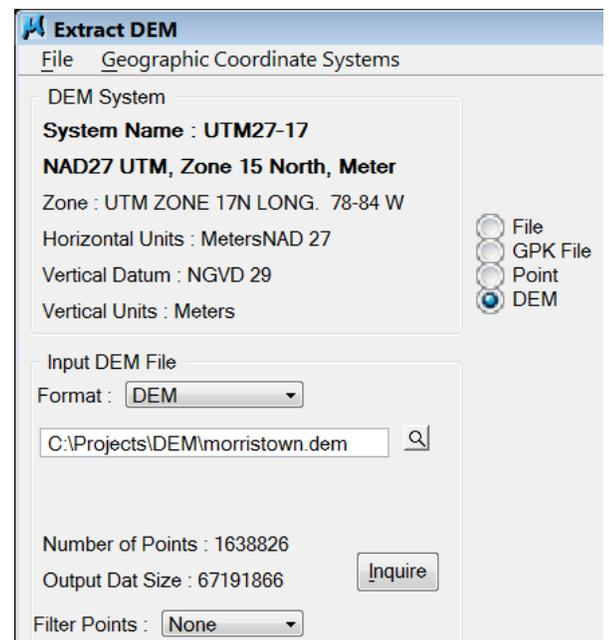
All quads west of longitude 90 degrees W should use Zone 15N and those east of 84 degrees west use Zone 17N. All of the rest of the state, which includes most of it, is covered by Zone 16N (84W – 90W).
