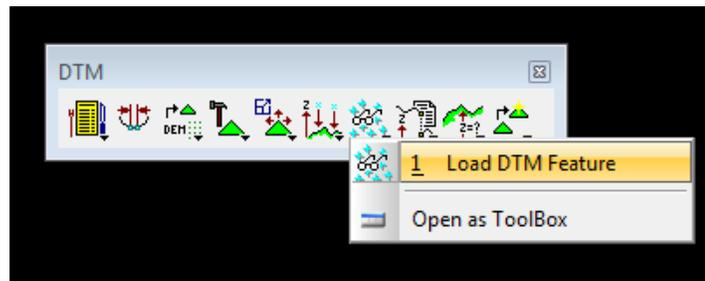
(18) In the **Load DTM Features** dialog, go to drop down option **File> Open** and go select **C:\Users\Public\Geopak Standards\tdotEXIST.Ipf** to load T.D.O.T. Design Division existing symbology settings.
