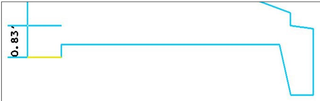
6. Change the distance to 2 feet in the Move/Copy Parallel. Copy the previous placed line up 2 feet. We now have the inside diameter of the pipe.
