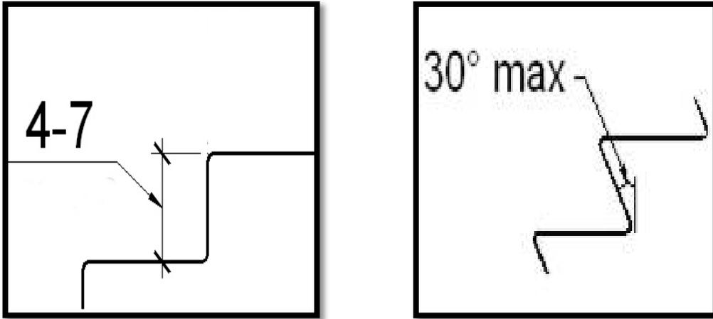
Figure 8 - Riser Height and Nosing Slope
