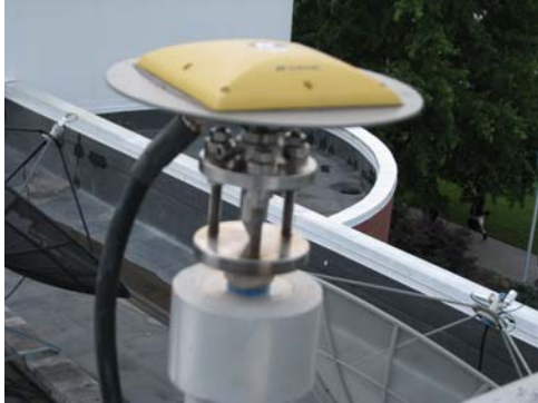
Antenna attached to monument
