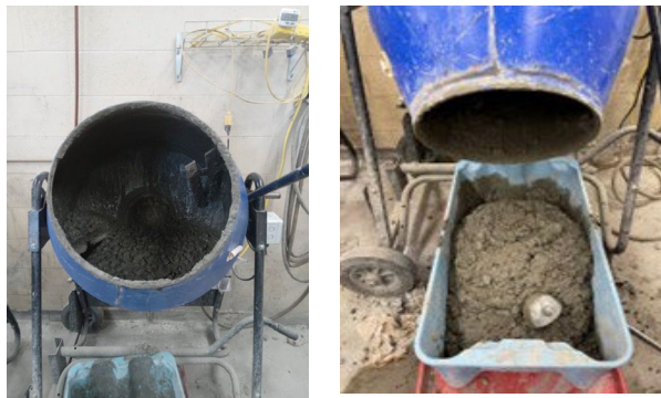
Figure 3-1 (a) Concrete drum mixer and (b) discharged concrete mix.
