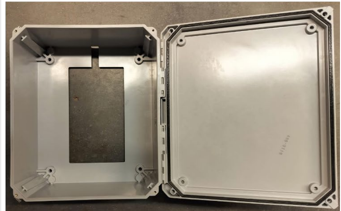
(b) Photo of the protective box for the tiltmeter.
