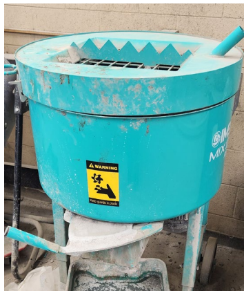
Figure 3-3 IMER 120 Plus high shear mixer.
