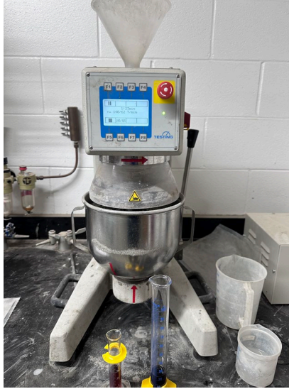
Figure 3-1 Planetary mixer used for small batch mixing.
