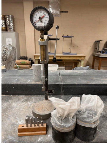
Figure 3-6 Setting time measurements with concrete penetrometer.
