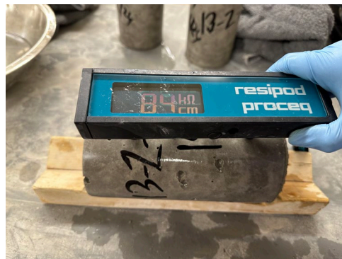
Figure 3-8 Example surface resistivity measurement with 4-point Wenner probe.
