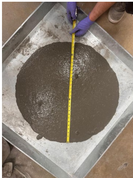
Figure 3-4 Slump flow measurement.
