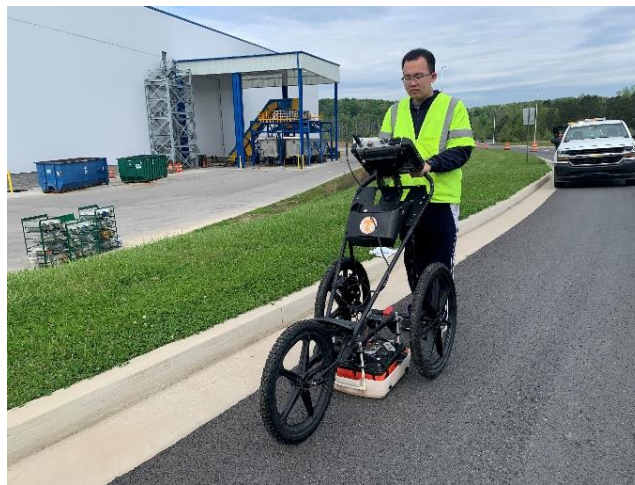
Figure 3-1. Pavement thickness detection process using GPR on the investigated pavement section in Chattanooga, TN.
