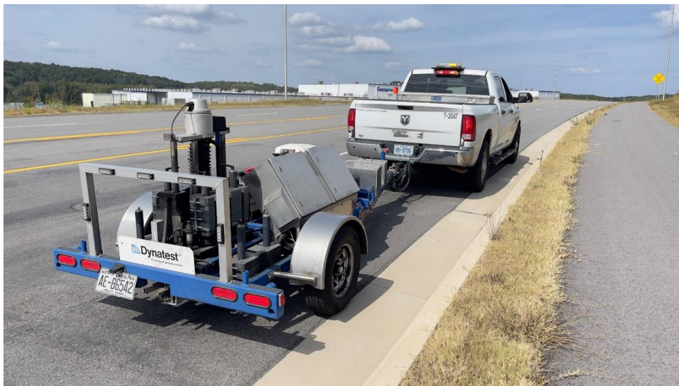
Figure 3-5. Fast Falling Weight Deflectometer (FFWD) setup.
