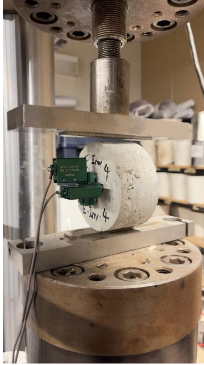
Figure 3-7. IDT Resilient modulus test setup.
