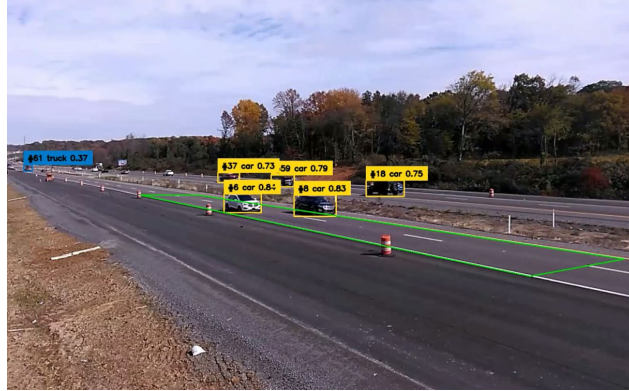
Figure 3-3 Sample of an image showing vehicles with their IDs and their bounding boxes.
