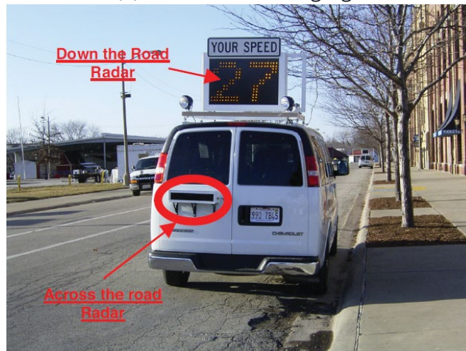
(b) SPE vehicle with radar and DMS
