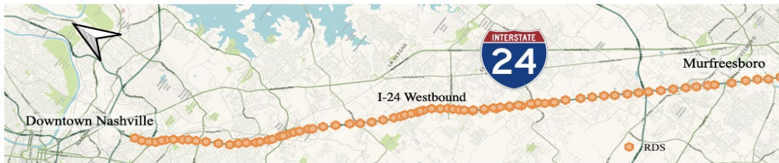
Figure 7: Layout of radar detection sensors along Interstate 24 near Nashville, TN. Source: Coursey et al., 2024
