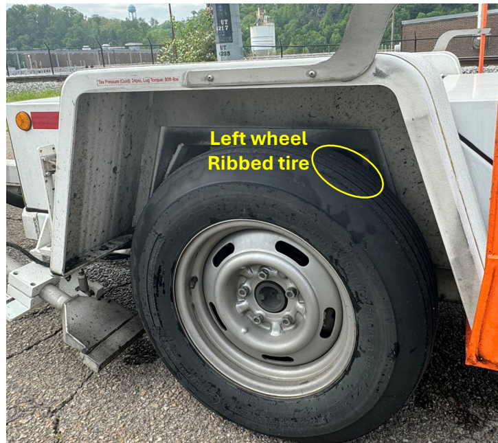
Figure 3-21 Tire configuration of the LWST.
