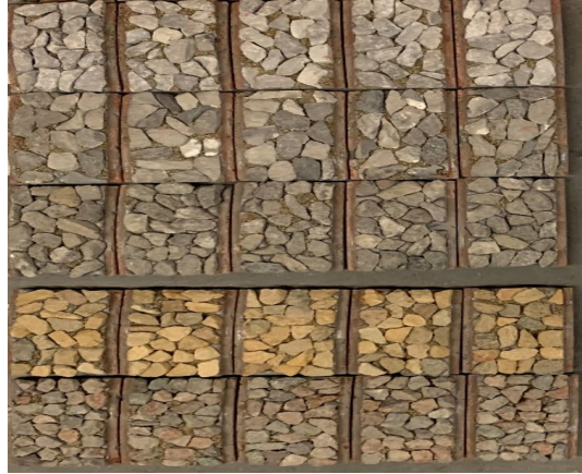
Figure 3-4 Aggregate coupons for frictional test.
