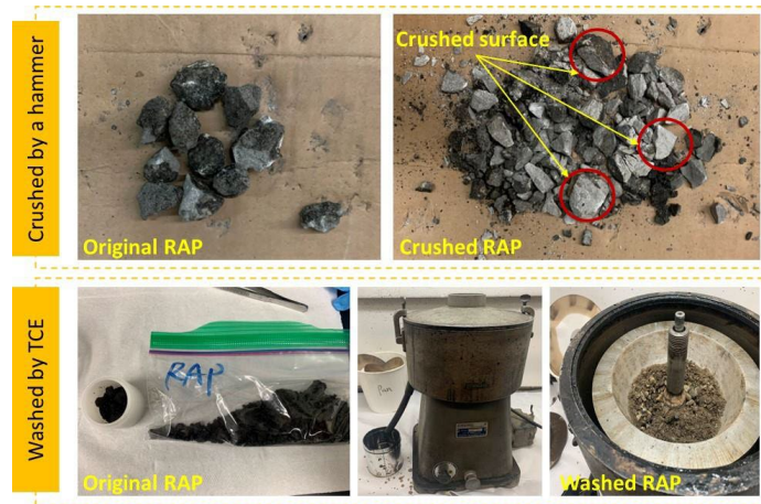
Figure 3-6 Processed RAP by hammer and TCE.
