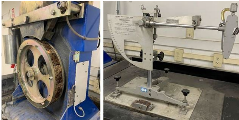
Figure 3-5 Polishing and testing of prepared aggregate coupons.
