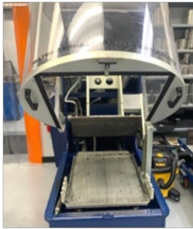
Figure 3-8 Heated asphalt roller compactor.
