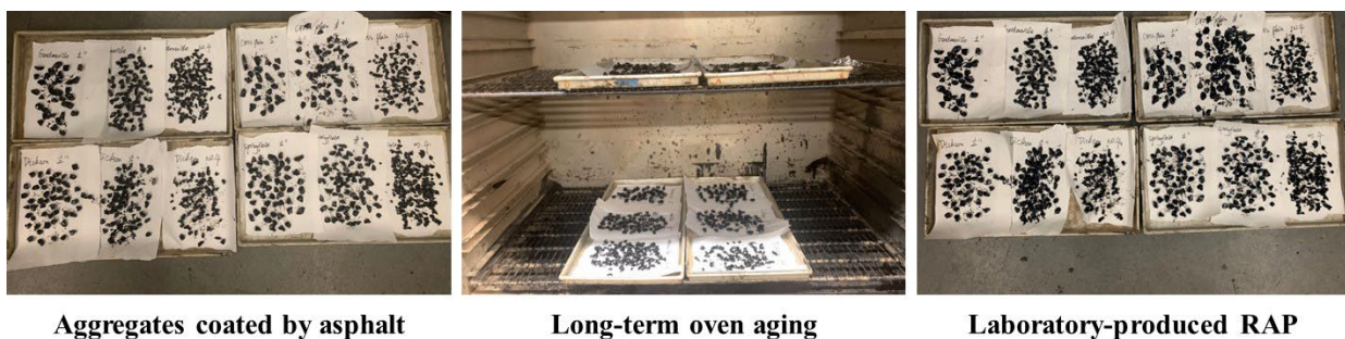
Figure 3-7 Laboratory preparation of RAP.
