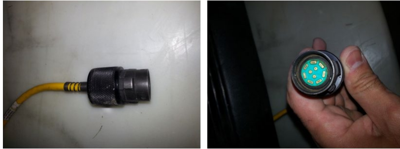
Figure 3-6. Data transfer cable from geode to geode, or from geode to software console on laptop
