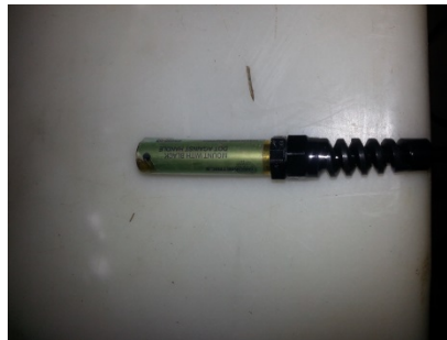
Figure 3-7. The trigger that attaches to the sledgehammer and signals the hit time
