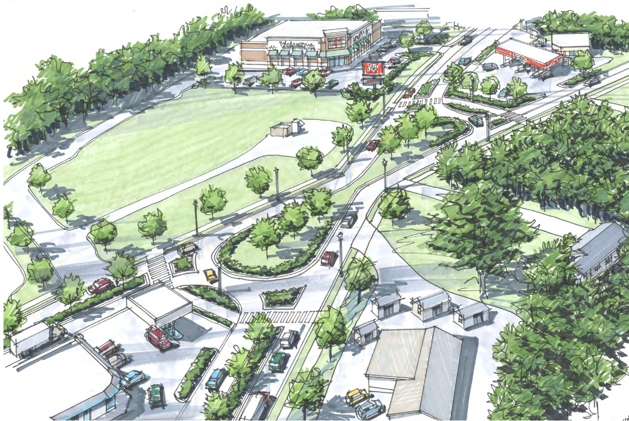
Figure 16: the peanut design will reduce conflict points at the intersection, increase safety and provide alternative means of transportation
