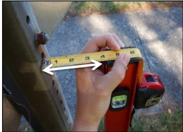
Example: Measuring sign leaning. 4 inches at the top of a 4-foot level = 1 inch per foot.
