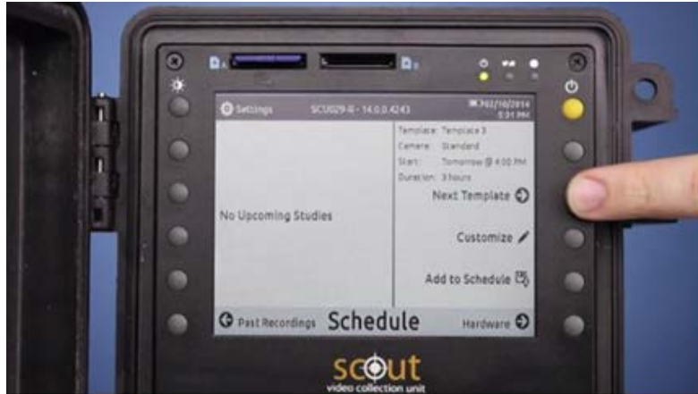
Figure 5.2: Miovision Scout (Traffic Counting Device)
