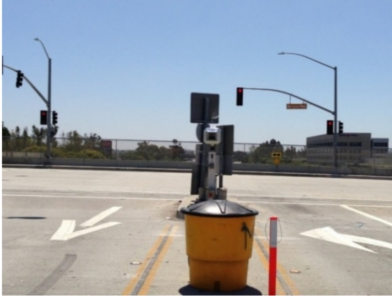
Figure 4.1: VODC Camera System
