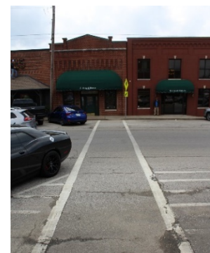
Figure 11: Transverse Lines Mid-Block Crossing
