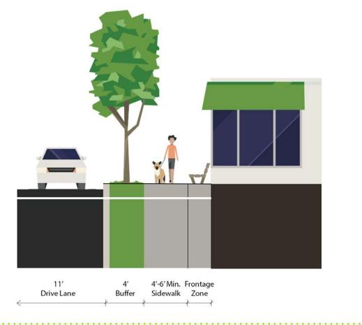
The pedestrian access route (sidewalk) should be at least four feet in width (preferably five to six feet) and kept clear of obstructions such as doors, table/benches, signs, and vegetation. The pedestrian access route is typically accompanied by a frontage zone adjacent to the building face, providing room for benches, cafe tables, lighting, and signage.
