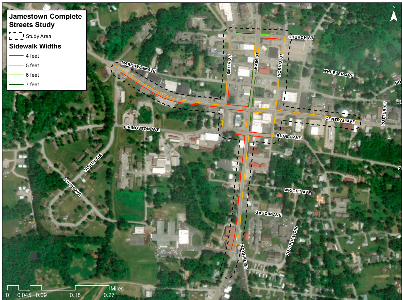
Figure 4-3. Updated Sidewalk Network Following Recommendations
