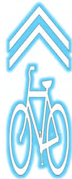
Shared Lane Marking
