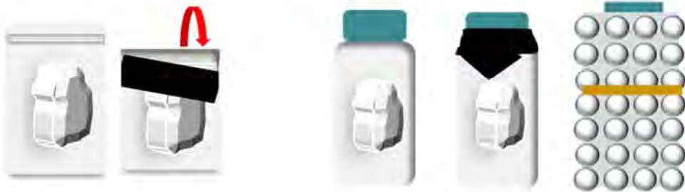
Seal in bag Tape bag seal (plastic thickness ≥4 mil)
