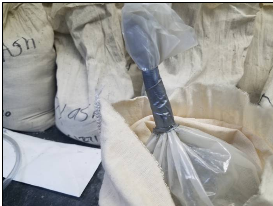
Figure 4: Sample bag with plastic liner tied separately with duct tape
