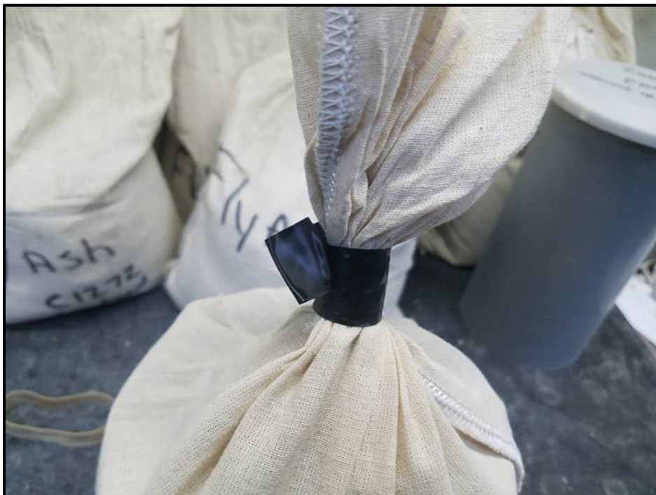
Figure 2: Sample bag tied with multiple wraps on electrical tape
