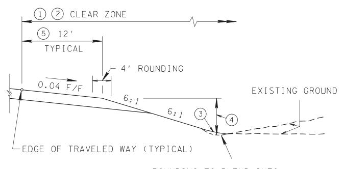
ROUNDING TO BLEND INTO EXISTING GROUND WHEN DITCH NOT REQUIRED FOR DRAINAGE.
