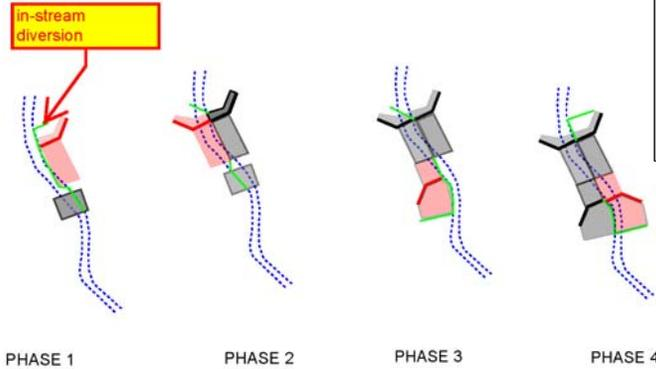
**SEQUENCE OF CONSTRUCTION FOR STR-1 CONCRETE BOX BRIDGE**
