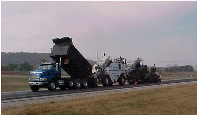
Use of shuttle buggy on thin overlay.
