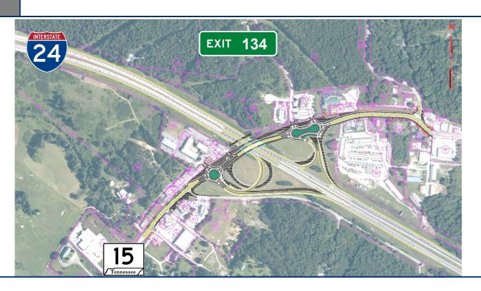
The project location and existing interchange configuration are contributing factors in anticipated challenges. The interchange is a partial cloverleaf with all ramps being on the east side, such that overhead bridge work that cannot be completed above live traffic is not easily detoured.
