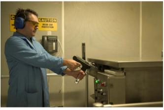
The Firearms Identification Unit's principal function is to determine if a bullet, cartridge case, or other ammunition component was fired from a particular weapon. The science of firearms identification extends beyond the comparison of bullets to include knowledge of the operation of all types of weapons, toolmark examination, the restoration of obliterated serial numbers on weapons and other evidence, the detection and characterization of gunpowder
