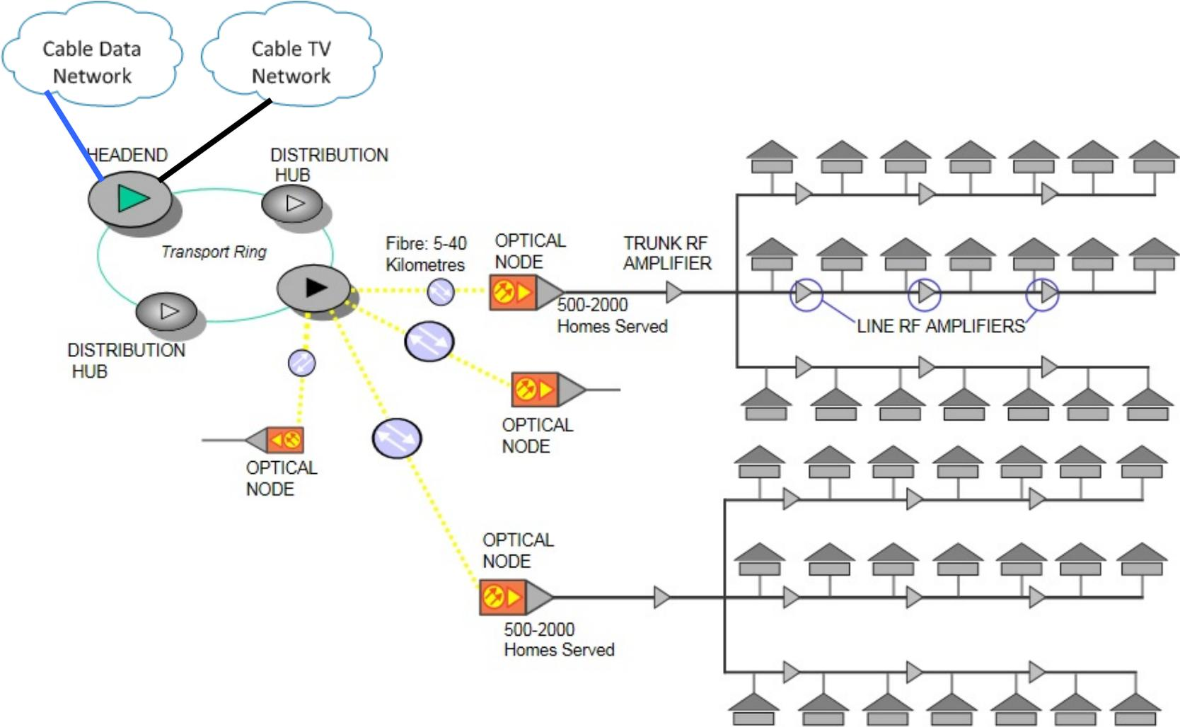
Diagram from Wikipedia "Hybrid Fibre-Coaxial"
