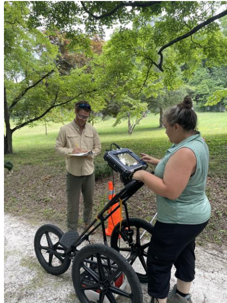
GPR Team Clearing the Site for Signage at the Bethel Cemetery.
