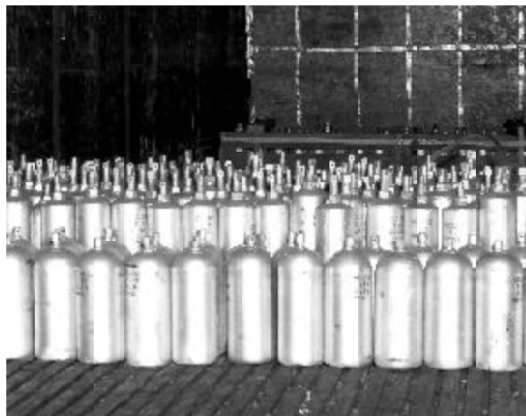
Flasks of mercury as received at the Y-12 Plant. About 24 million pounds of mercury were used.
