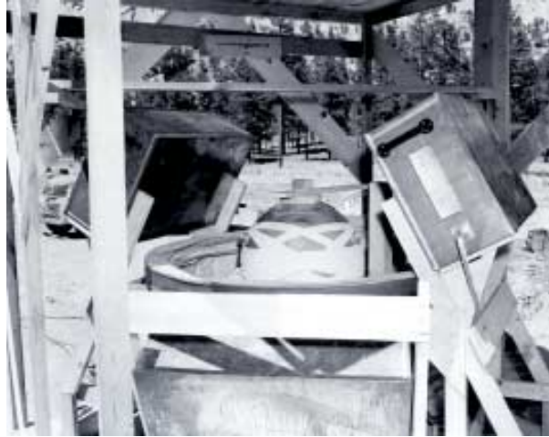
A Los Alamos apparatus that used RaLa to test the implosion process in early atomic weapons. A lanthanum radiation source was placed inside the sphere shown in the center of this photo.
