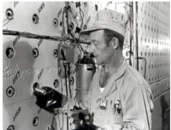
Uranium fuel slugs, such as these being loaded into the Clinton Pile, were used as the source of barium for RaLa production.
